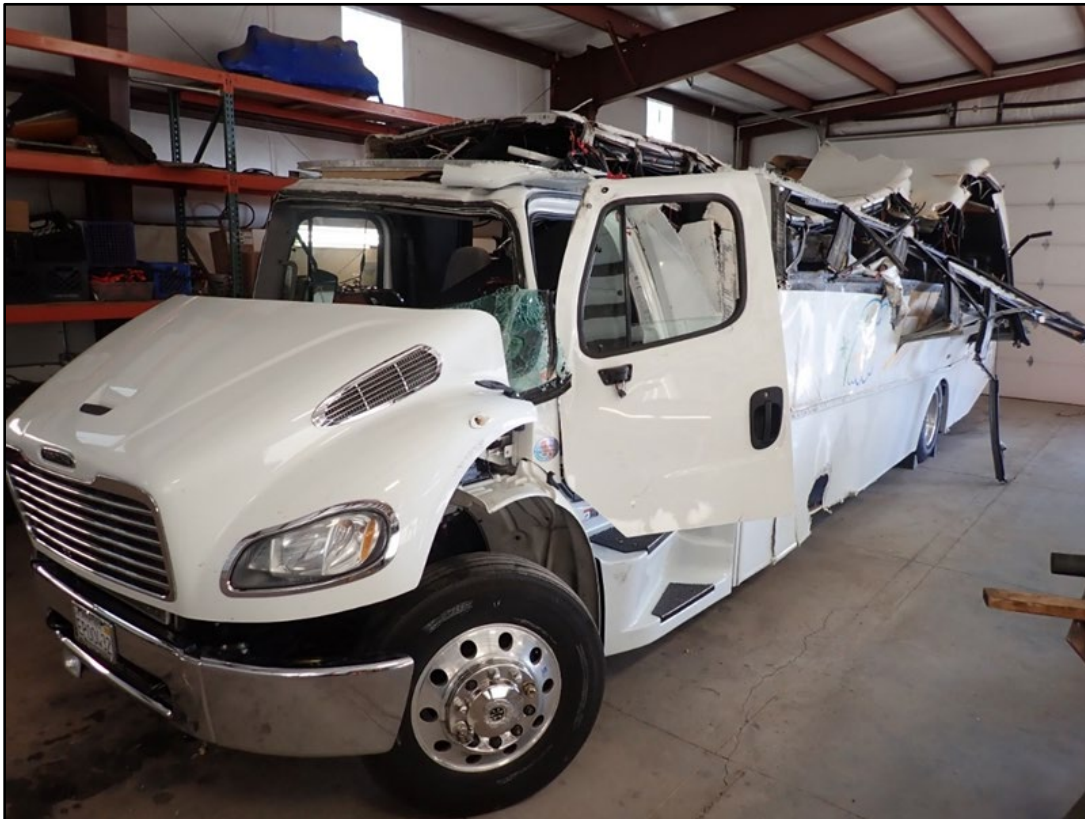
Figure 10. Damage on left side of bus.
