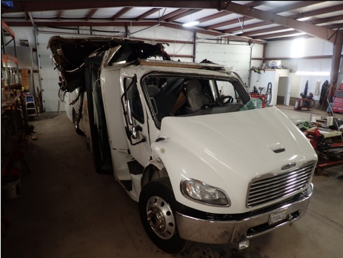
Figure 11. Damage on right side of bus.
