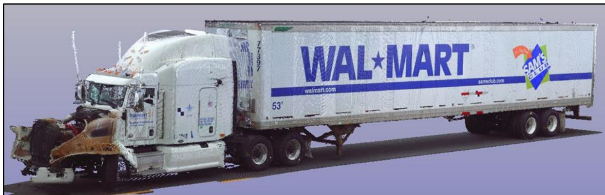
Figure 4. Three-dimensional scan image showing damage to the Walmart Transportation truck from the driver side.
