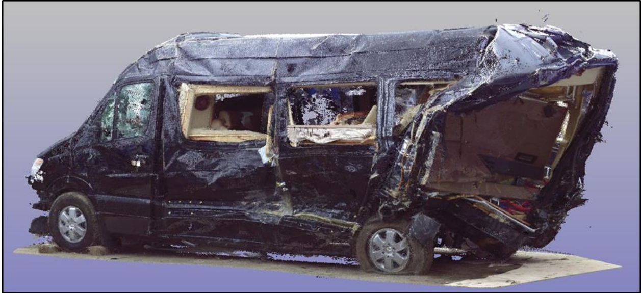
Figure 7. Three-dimensional scan image showing damage to the limo van from the driver side.
