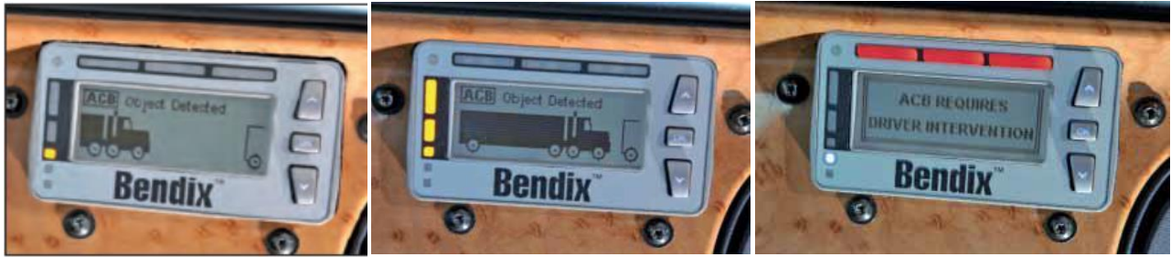
Figure 6. In-cab displays of Bendix Wingman ACB system alerts showing a following distance alert, a stationary object alert, and an impact alert. (Image source: Bendix system operator’s manual [Bendix 2010].)
