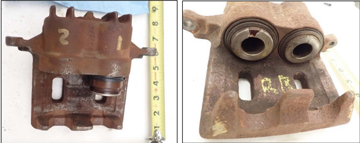
Figure 20. Photographs of brake calipers, postcrash. Left photo shows left rear brake caliper with one piston extruding from piston bore. Right photograph shows right rear brake caliper with both pistons seated within piston bores.
