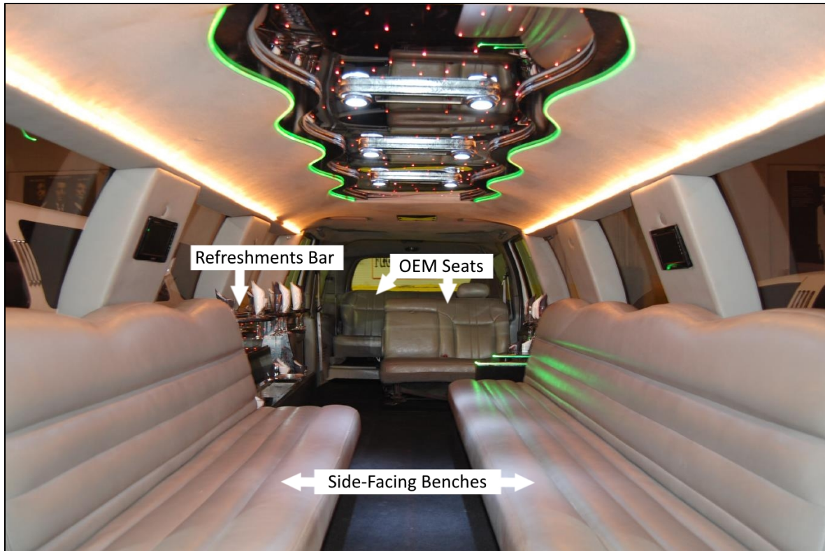
Figure 16. Photograph of limousine's interior, looking from front of vehicle toward rear of passenger compartment. (Source: Advantage Transportation Group, 2010)
