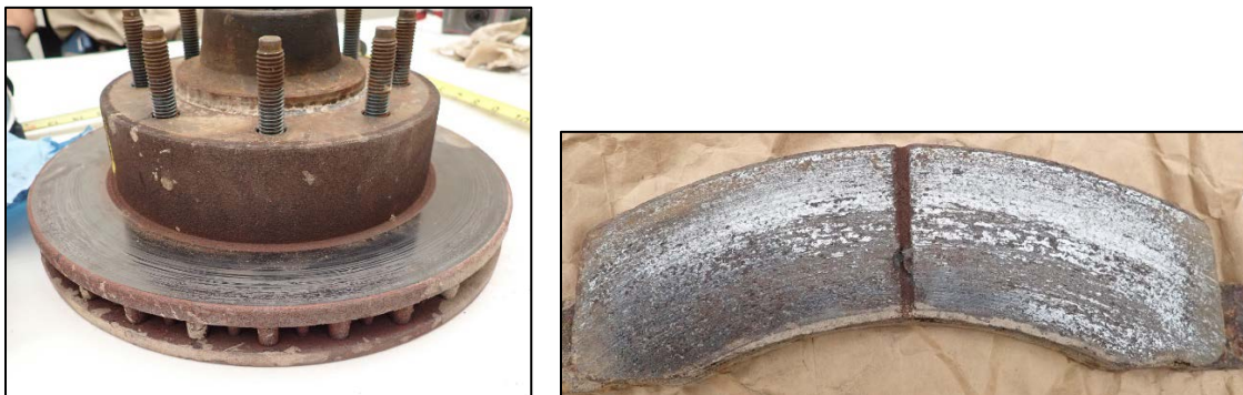
Figure 21. Photographs of right front disk brake rotor and inner right front brake pad surface. Left photo shows right front disc brake rotor with corrosion and swept surfaces. Right photo shows the inner right front brake pad surface with corrosion and uneven wear patterns, glazing, and deterioration.
