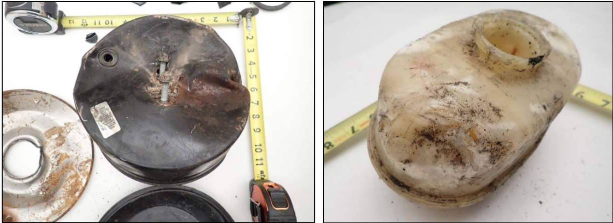
Figure 18. Photographs of brake components, postcrash. Left photo shows damaged power brake vacuum booster. Right photo shows damaged plastic brake fluid reservoir. (Source: NYSP)
