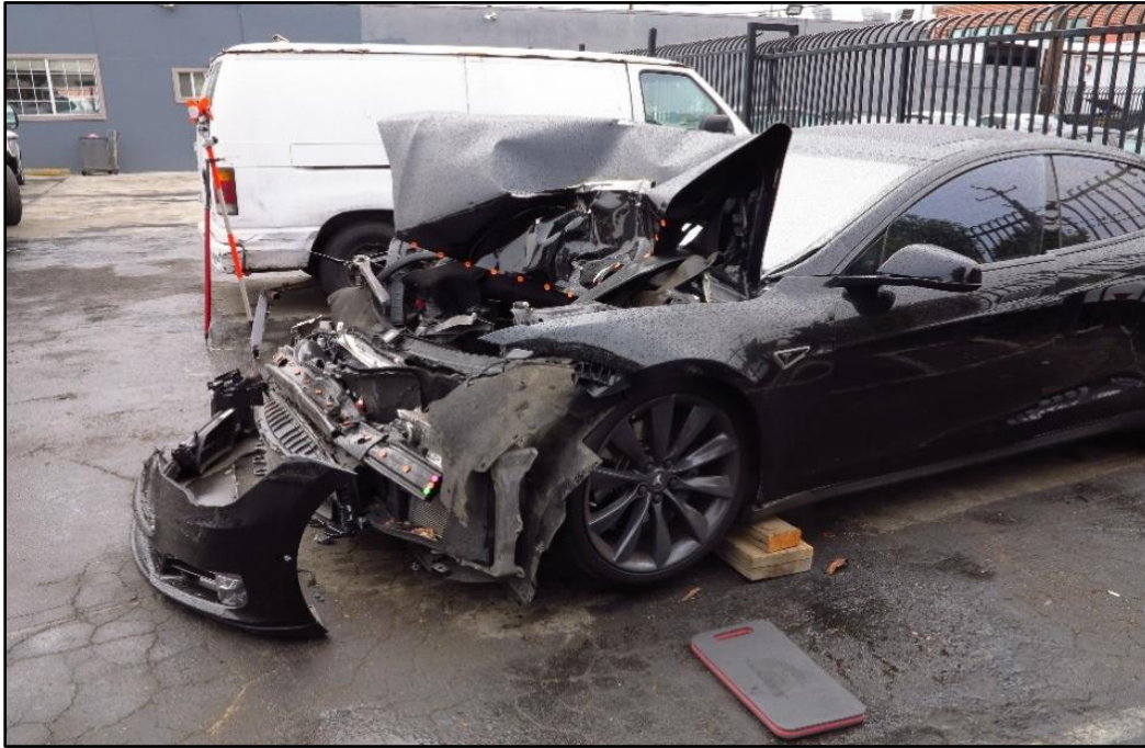
Figure 3. Front-end crash damage to Tesla.
