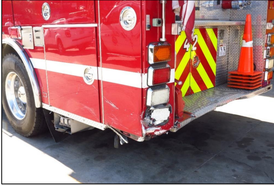
Figure 4. Crash damage to rear deck and left rear corner of fire truck.
