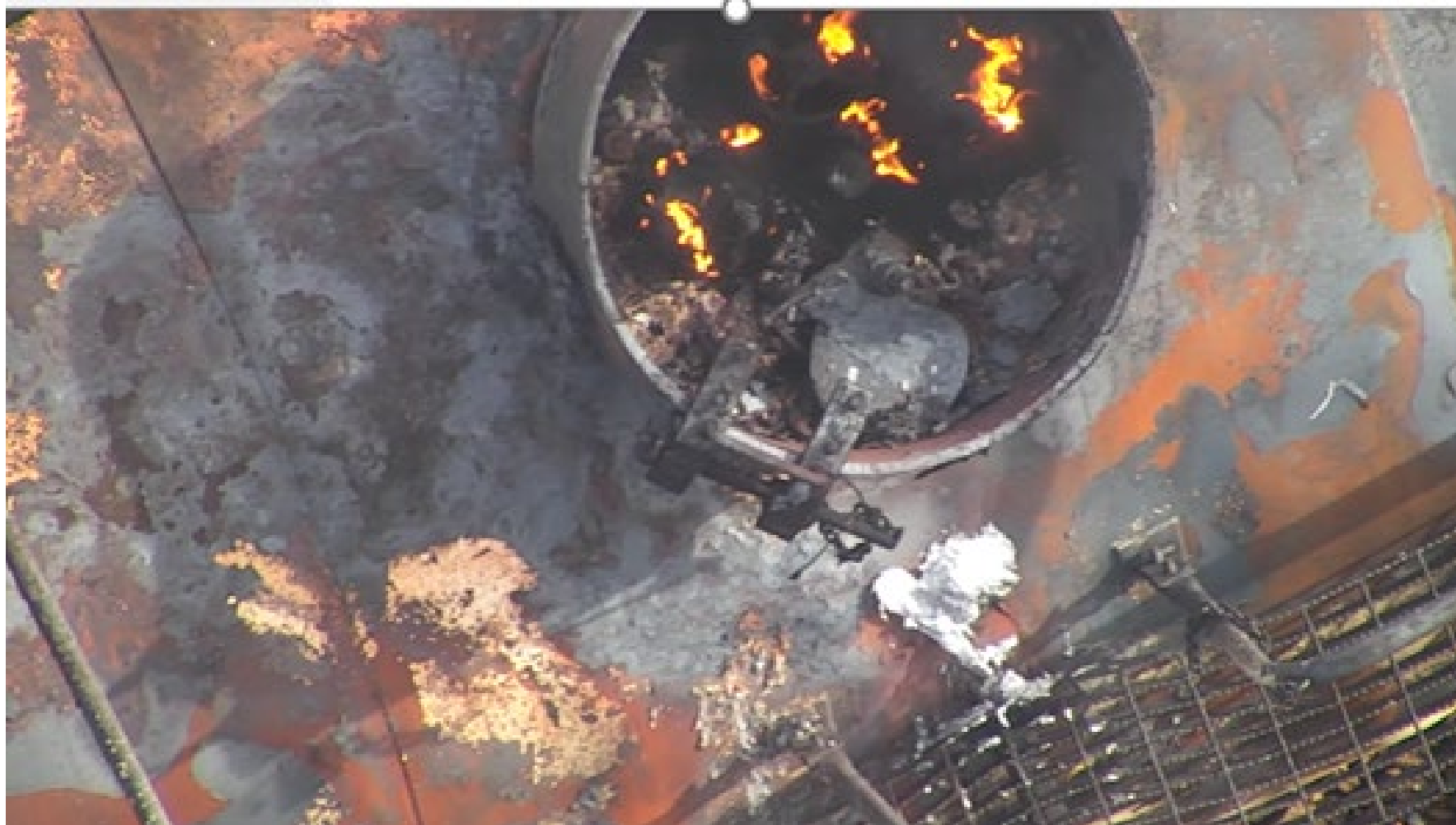
Cars 28, 29, 53 (Vinyl chloride Cars) PRD, Fire Inside Housings
