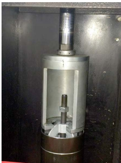
Figure 8-2 Loosen Locknut and Compress Valve Spring
