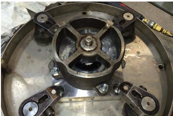
Figure 7-2 Fill with Water; Observe Pressure Gauge and Bubbling
