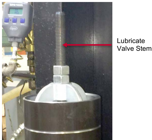
Figure 8-1 Remove Wire Seal and Lubricate Valve Stem
