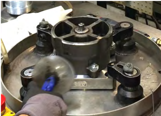
Figure 8-5 Blow Away Remaining Liquid and Install Seal Wire
