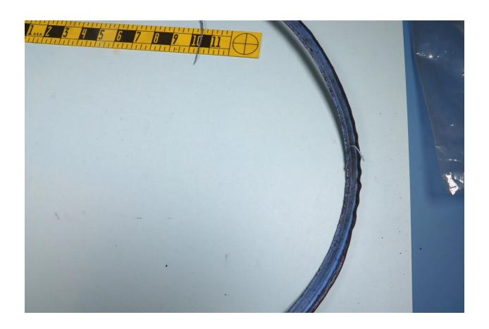
2. OCPX80235 pressure relief device gasket, recovered during valve tear down at TrinityRail Car Repair, 2850 Peden Rd., Saginaw, Texas, March 15, 2023.
