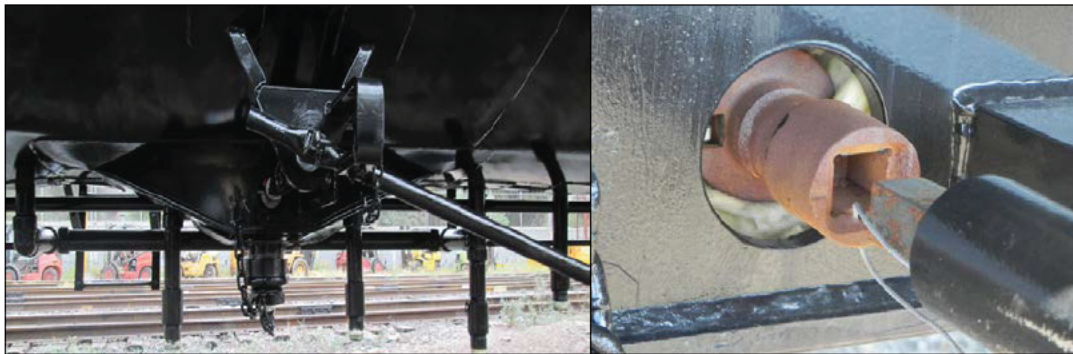
DOT-117 BOV valve and removable handle
