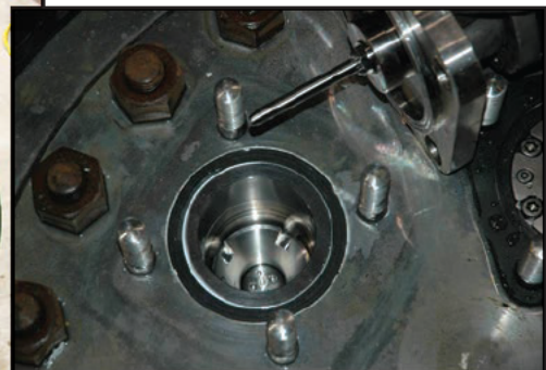
New valve arrangement for Chlorine and other service
