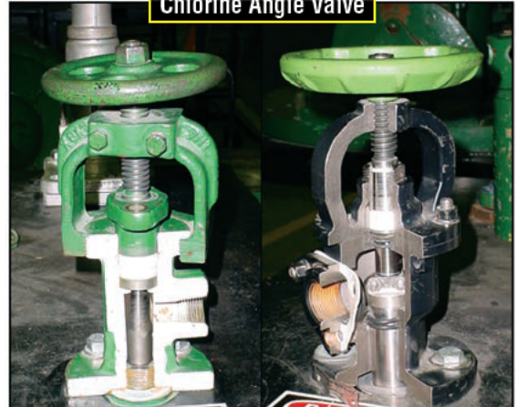
Chlorine Angle Valve
