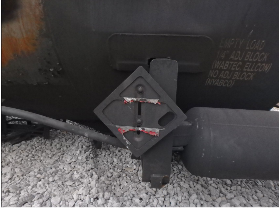
The above photo was taken by an NTSB investigator at the accident site. At the center of the photo is a placard holder. A charred red material is wrapped around the crossbars of the placard. No placard text is visible.
