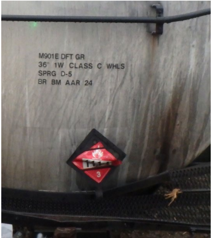
The above photo was taken by an NTSB investigator at the accident site. At the center of the photo is a placard holder. A charred red material is wrapped around the crossbars of the placard. No placard text is visible.
