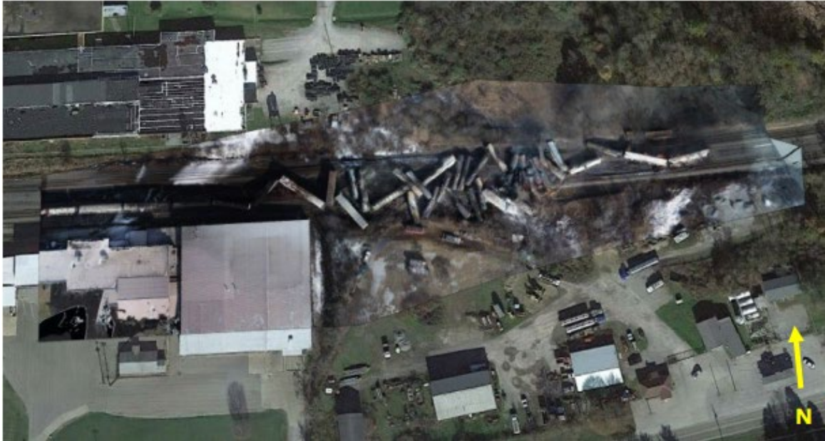
Figure 1: Overhead view of the Norfolk Southern Railway's train derailment with hazardous materials release in E. Palestine, OH. This is an orthomosaic image overlaid atop Google Earth, as developed by NTSB's UAS Aerial Imagery Specialist/RPIC, Eric Gregson and presented in the Unmanned Aircraft System Aerial Imagery Specialist's Field Notes.
