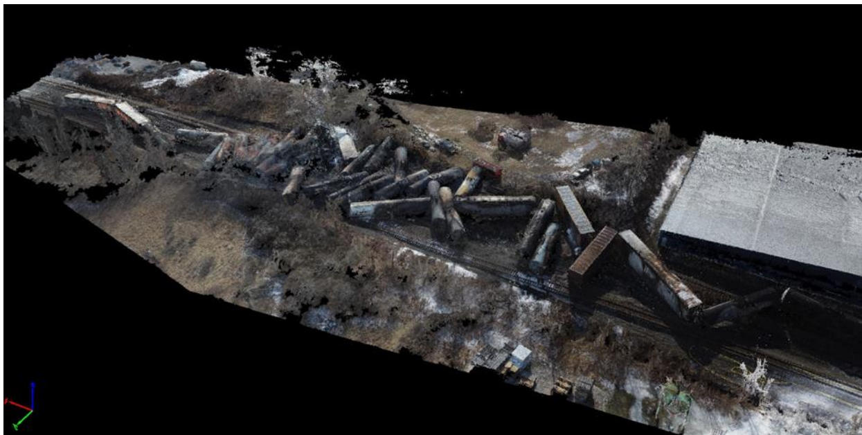
Figure 4. Generated Point Cloud of the main derailment site.
