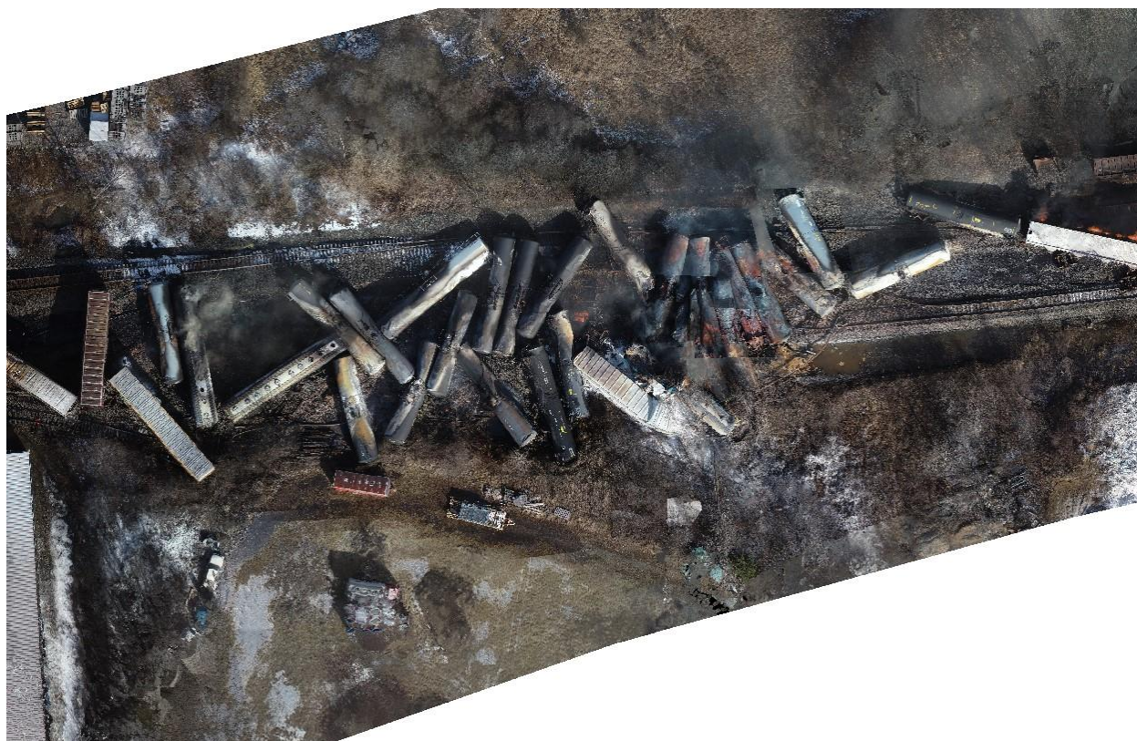
Figure 3. Generated Orthomosaic Image of the main derailment site.
