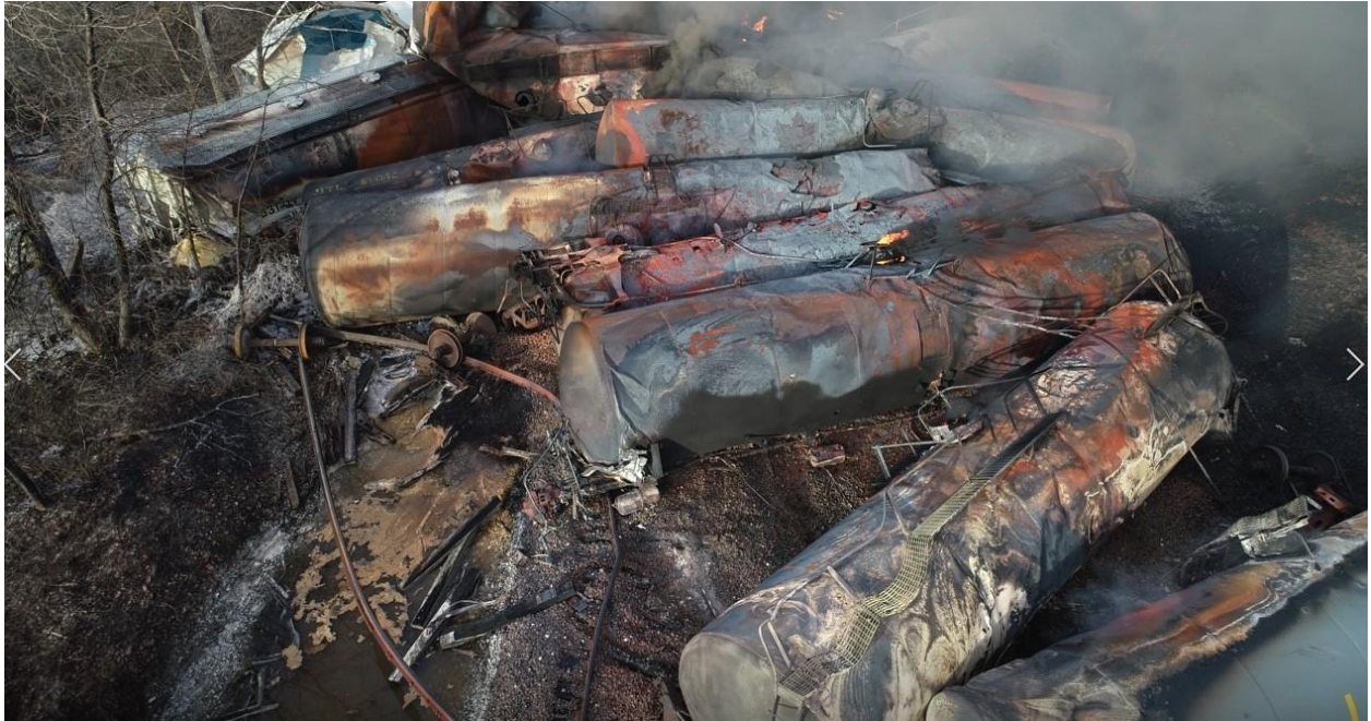
Figure 2. Image from video flight showing the resting positions of several tank cars.
