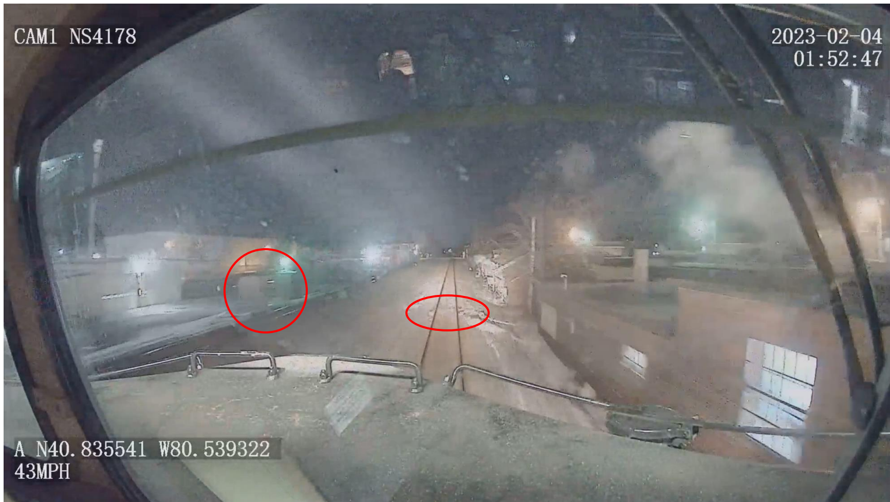
Figure 2. View as the train approached the alerting hot box detector, with the detector visible on the tracks and the equipment shed visible to the left.
