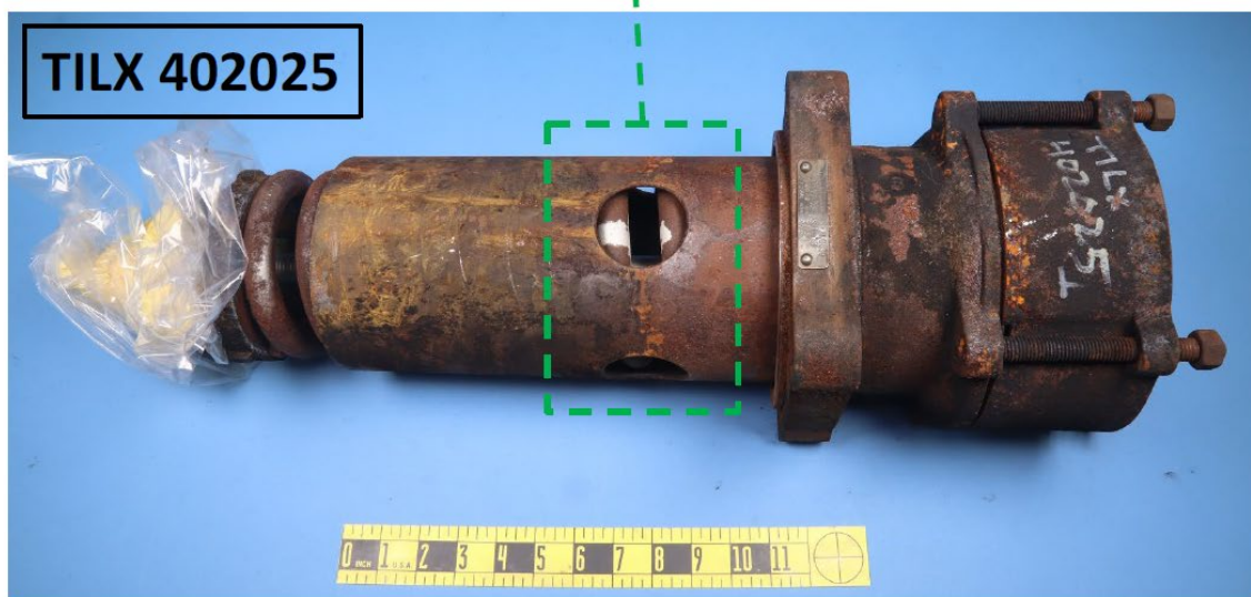
Figure 1. Overall and close-up photos showing the PRD from tank car TILX 402025. The red arrow points to the approximate location XRF measurements were taken in a silver-colored area exposed after bead-blasting removed the dark colored soot and debris on the valve spring.
