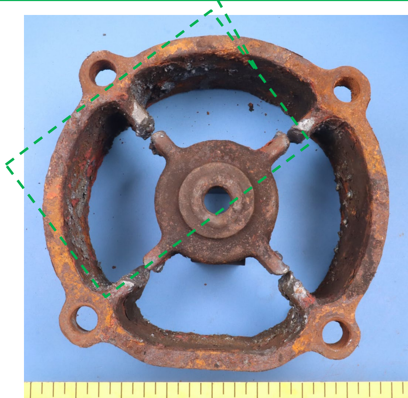
Figure 4. Macro (bottom) and close-up (top) photos showing the top guide pieces of the PRD as viewed from the outboard side.
