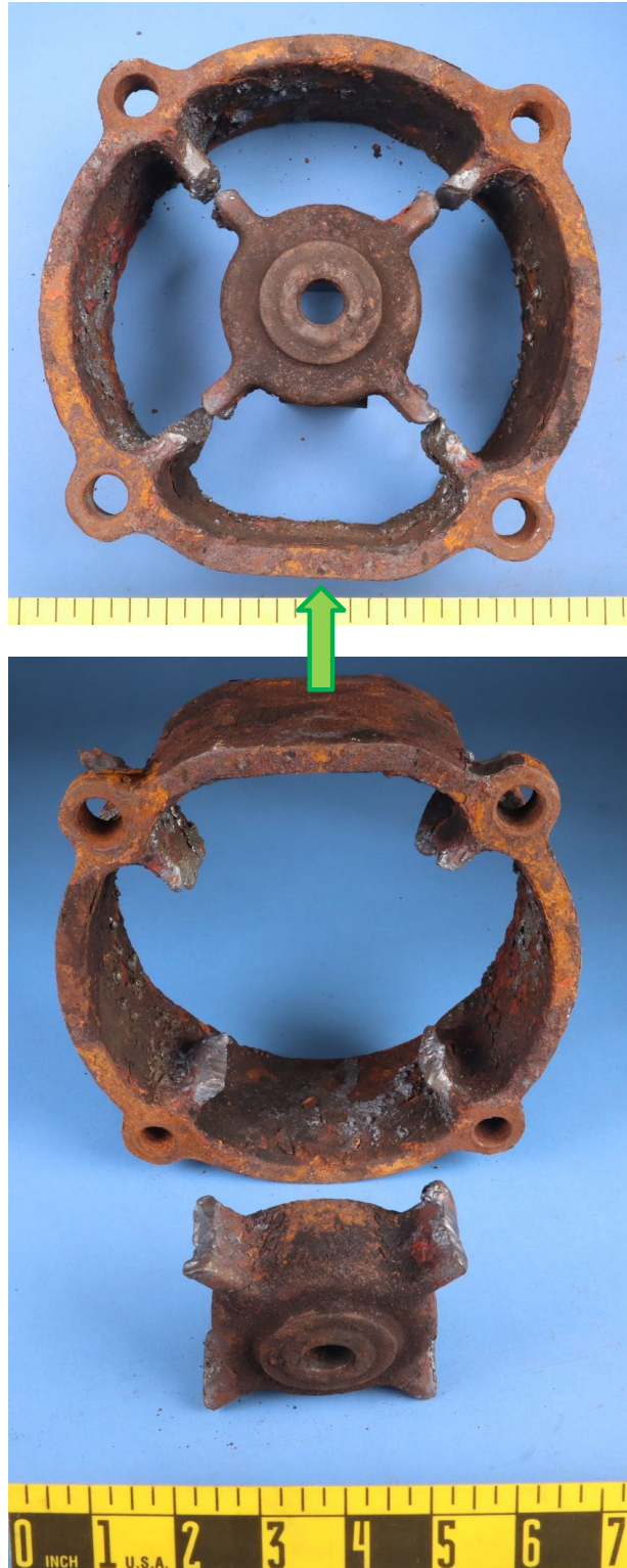
Figure 3. Macro photos showing the top guide pieces of the PRD as viewed from the outboard side.
