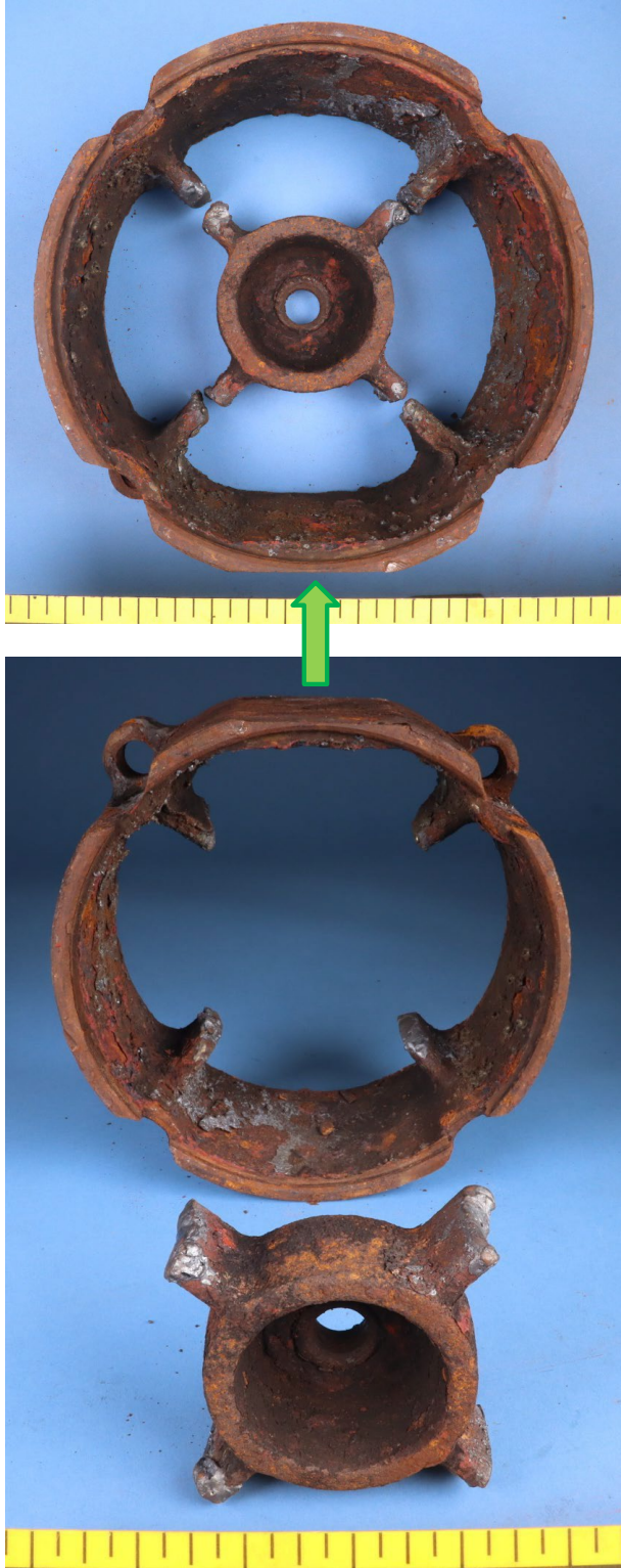
Figure 5. Macro photos showing the top guide pieces of the PRD as viewed from the inboard side.
