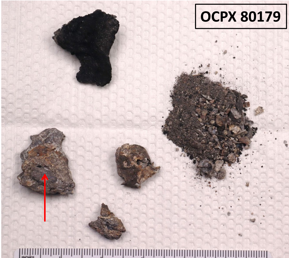
Figure 2. Macro photo showing the sample collected from rail car OCPX 80179 while on-scene. The red arrow points to the approximate location XRF measurements were taken on the piece of debris chosen for analysis.
