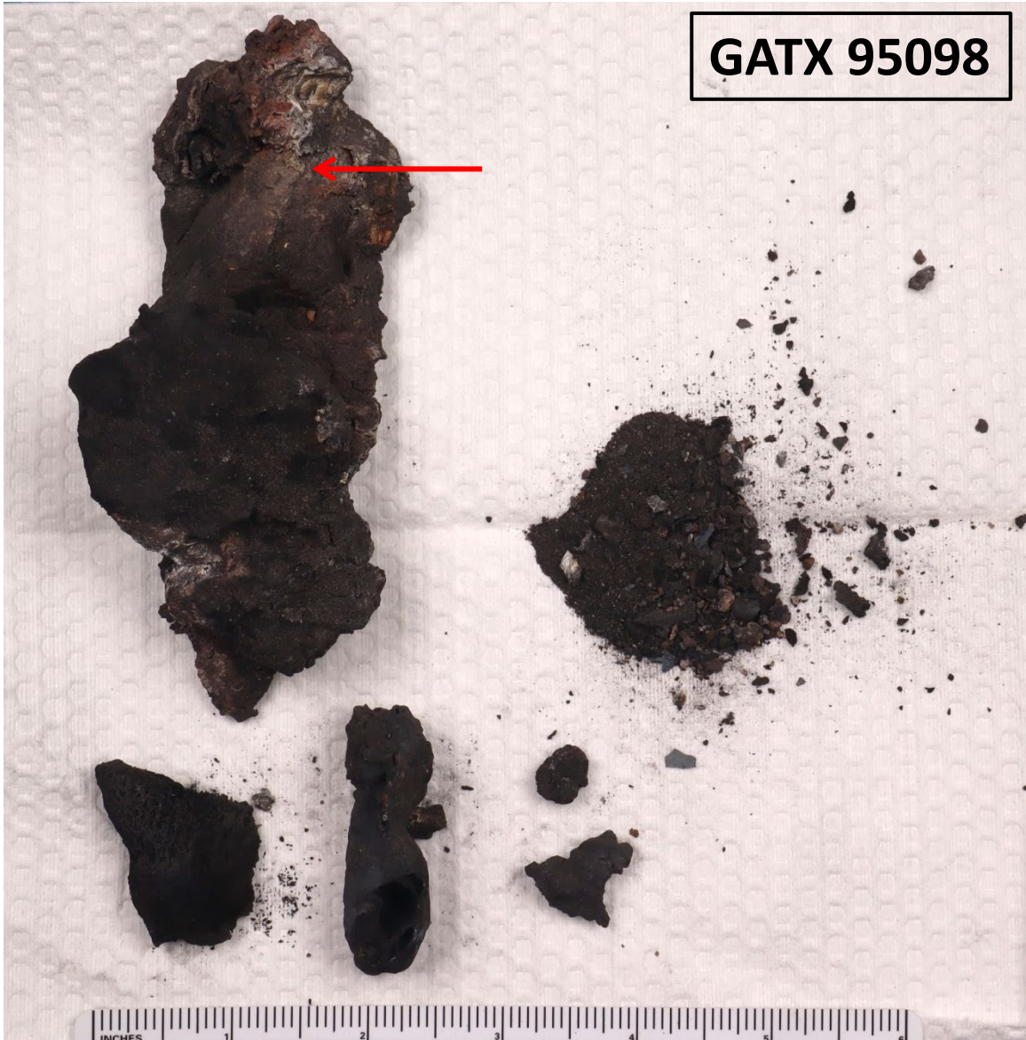
Figure 3. Macro photo showing the sample collected from rail car GATX 95098 while on-scene. The red arrow points to the approximate location XRF measurements were taken on the piece of debris chosen for analysis.
