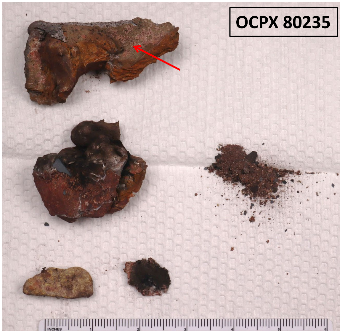
Figure 1. Macro photo showing the sample collected from rail car OCPX 80235 while on-scene. The red arrow points to the approximate location XRF measurements were taken on the piece of debris chosen for analysis.
