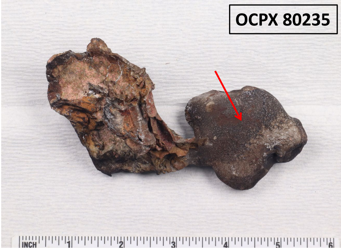
Figure 4. Macro photo showing the sample collected from rail car OCPX 80235 during PRD testing. The red arrow points to the approximate location XRF measurements were taken on the piece of debris chosen for analysis.
