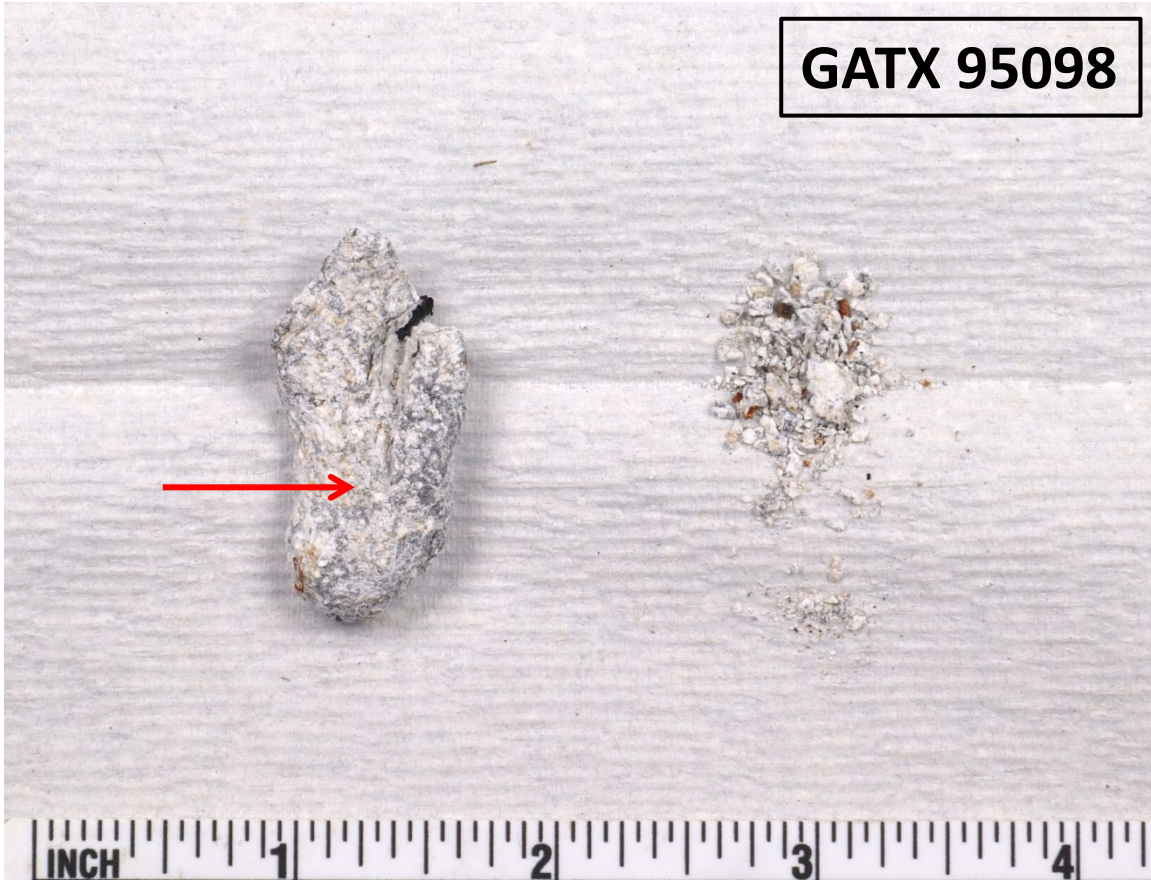
Figure 5. Macro photo showing the sample collected from rail car GATX 95098 during PRD testing. The red arrow points to the approximate location XRF measurements were taken on the piece of debris chosen for analysis.
