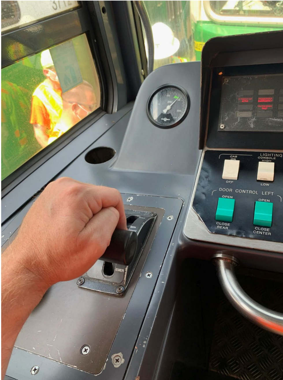
Figure 6: Exemplar operator engaging the master controller. Source: NTSB
