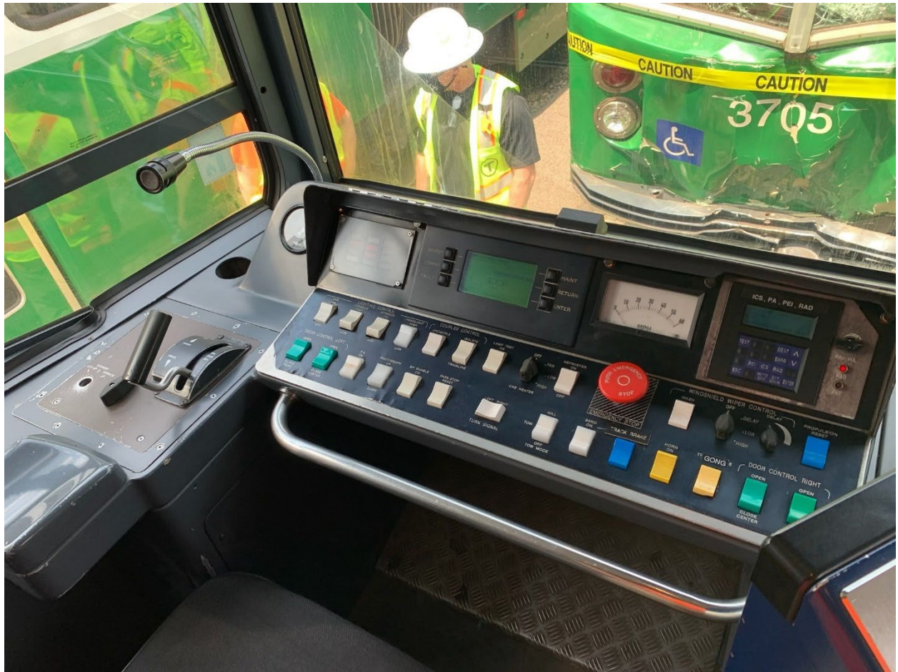
Figure 3: Photo of operator console. Source: NTSB
