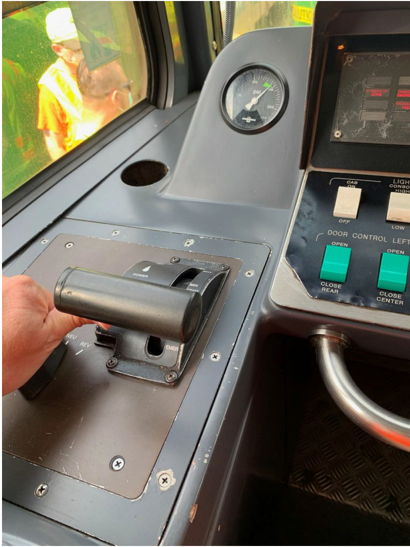
Figure 5: Master Controller in operating position, power and brake can be engaged, “deadman” switch engaged. Source: NTSB
