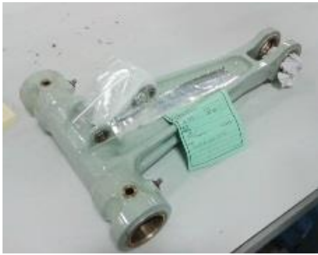
Figure 35 As-Received Upper Drag Brace
