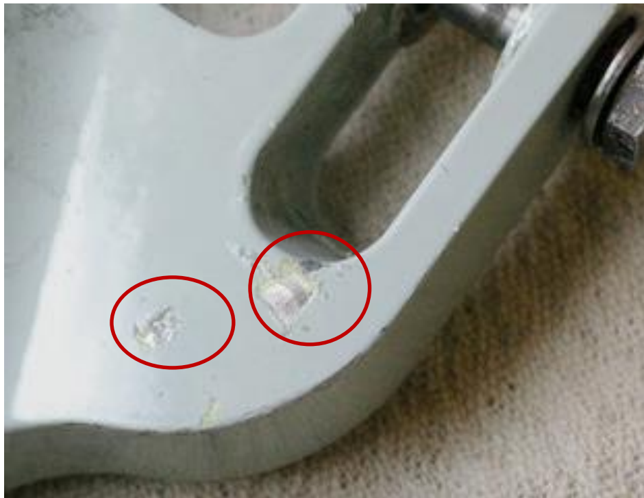
Figure 10 Contact Damage from Contact with the end of the Drive Arm Assembly
