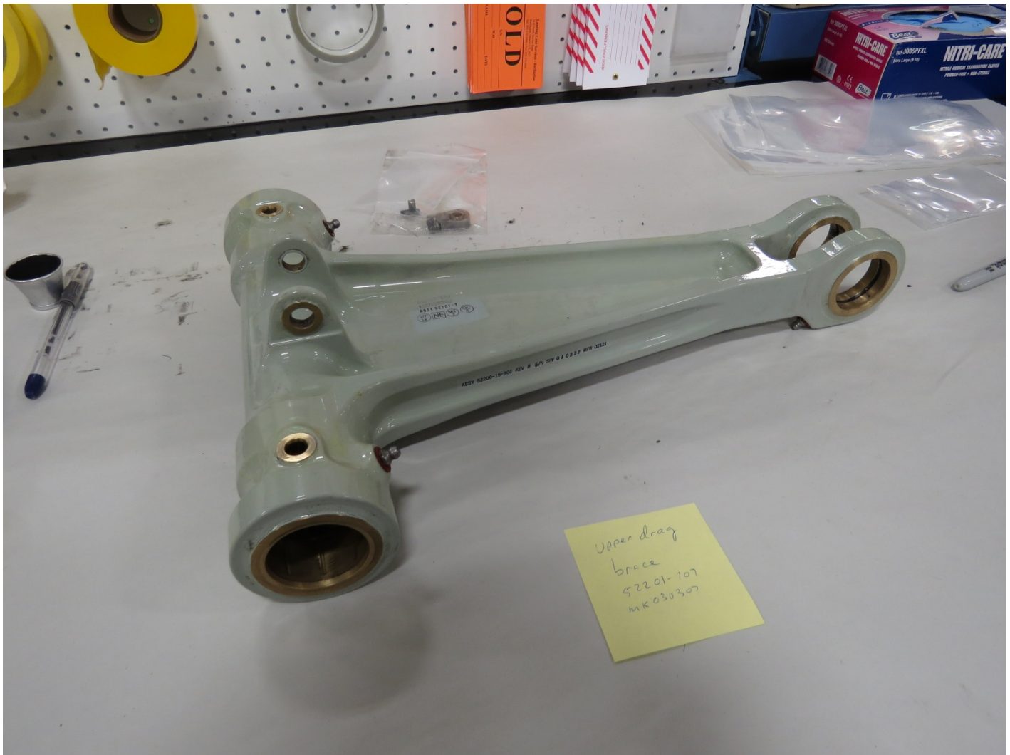
Figure 14 Upper Drag Brace
