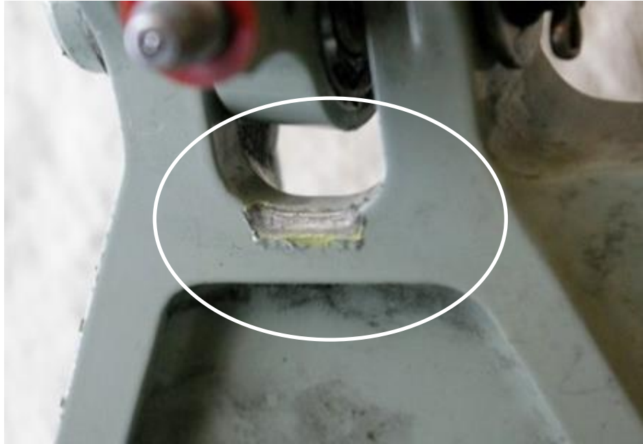
Figure 9 Impact Damage from Contact with the Upper Link Assembly
