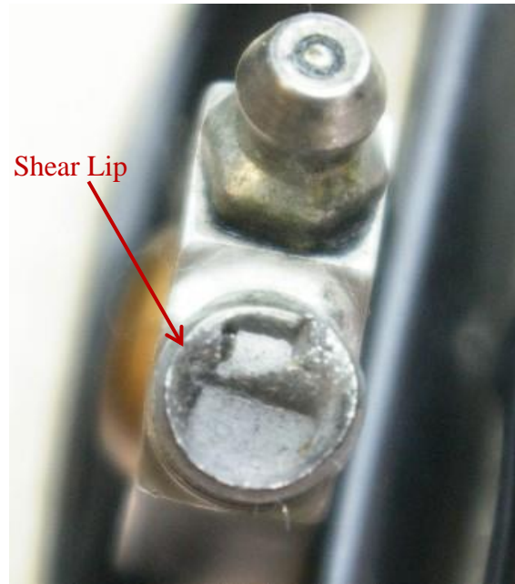
Figure 15 Spherical Bearing Fracture Face
