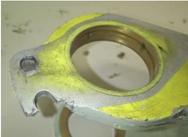
Figure 28 Fractured Lug Hole and Adjacent Damage
