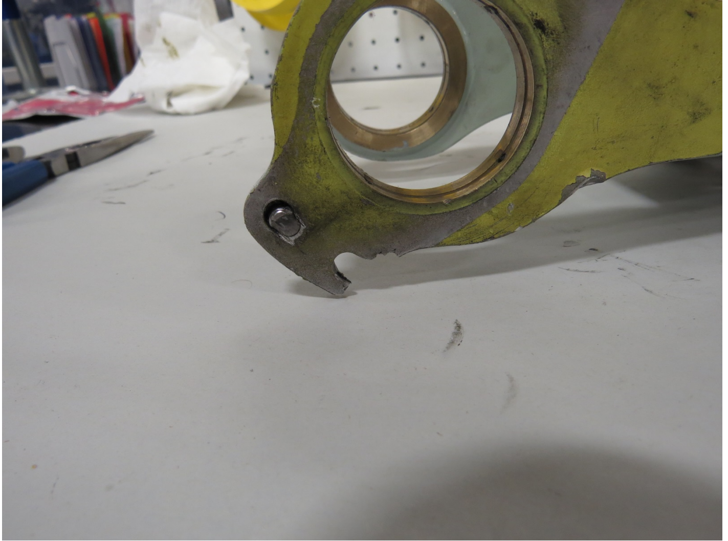
Figure 10 Sheared off anti-rotation bolt in lower bolt hole
