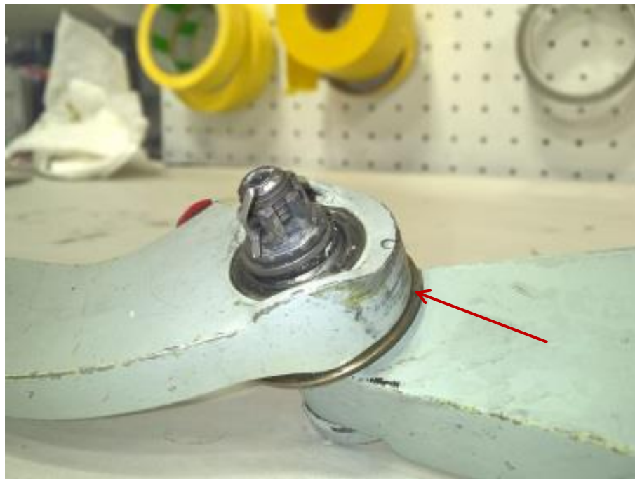
Figure 13 Circumferential Paint and Primer Scrapes on end of Drive Arm Link
