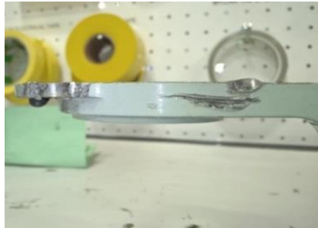
Figure 29 Gouging and Impact Damage
