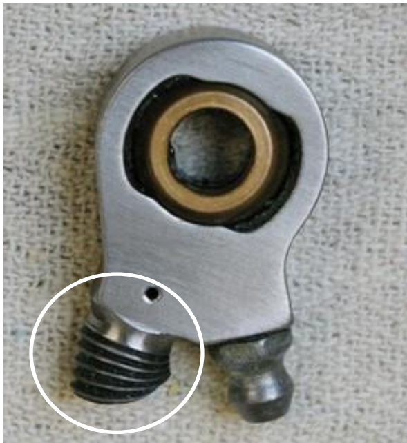
Figure 14 Fractured Spherical Bearing
