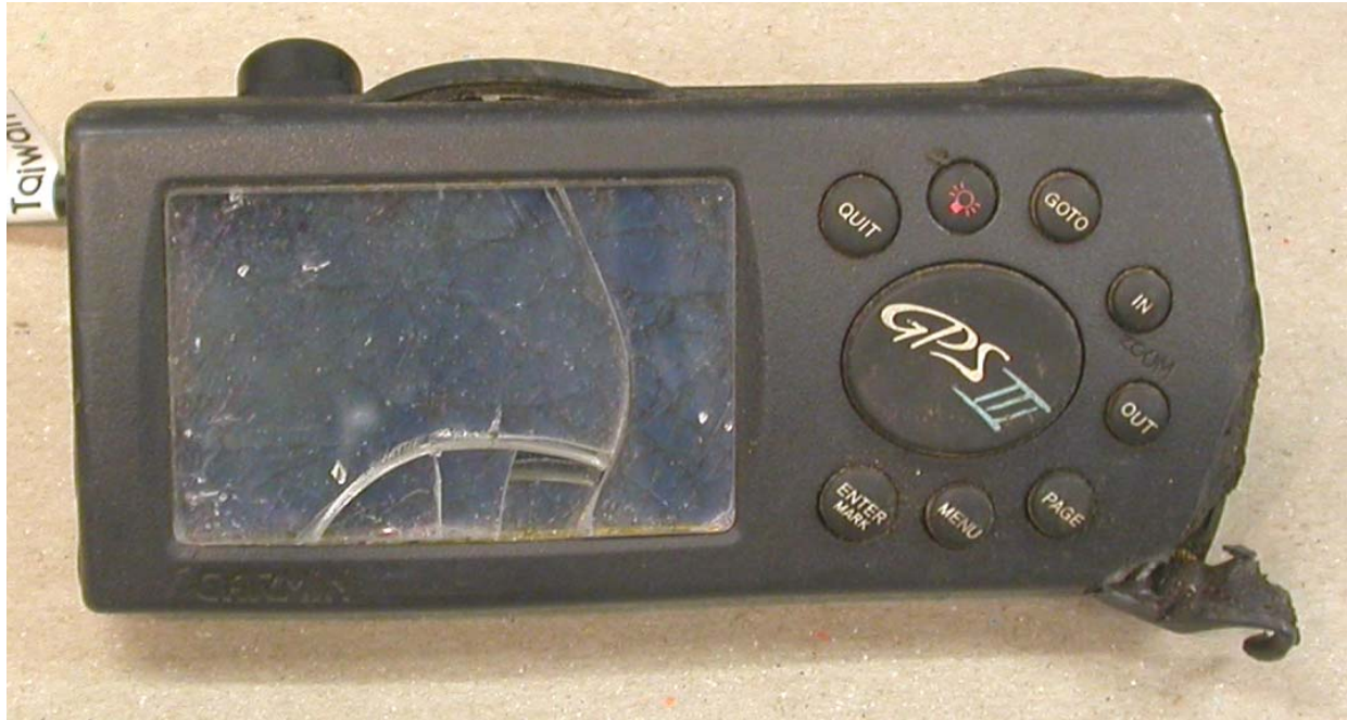
Figure 1. External front view of the Garmin GPS III Pilot (s/n 40903064) showing signs of impact damage to the outer case and display.
