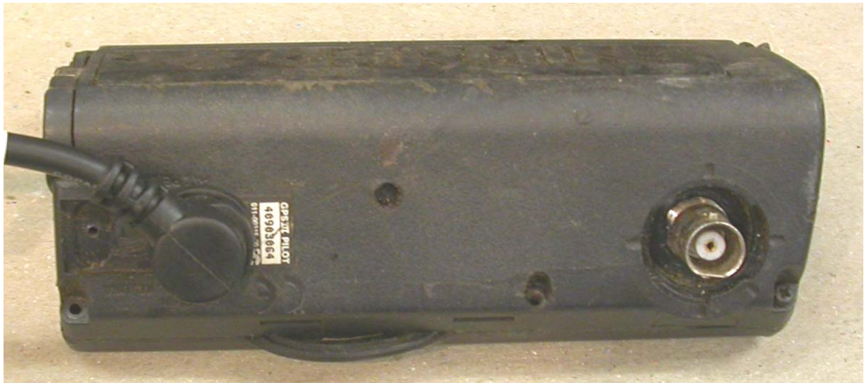
Figure 2. External rear view of the Garmin GPS III Pilot (s/n 40903064) showing signs of impact damage to the outer case and display.
