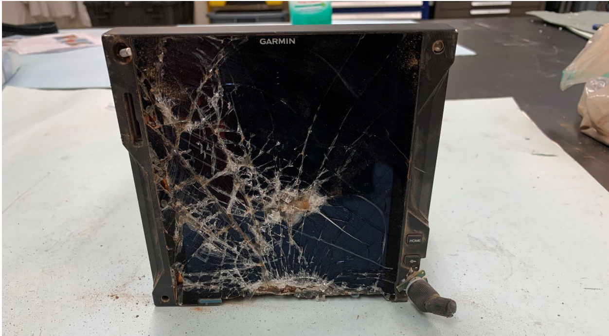
Figure 1. Photo of the GTN 750Xi showing impact damage.
