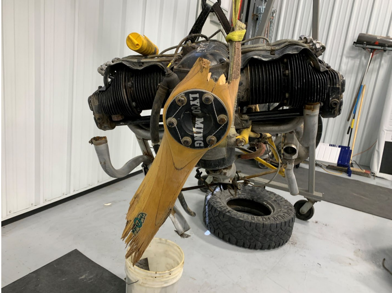
Figure 6. View of damaged engine and propeller.
