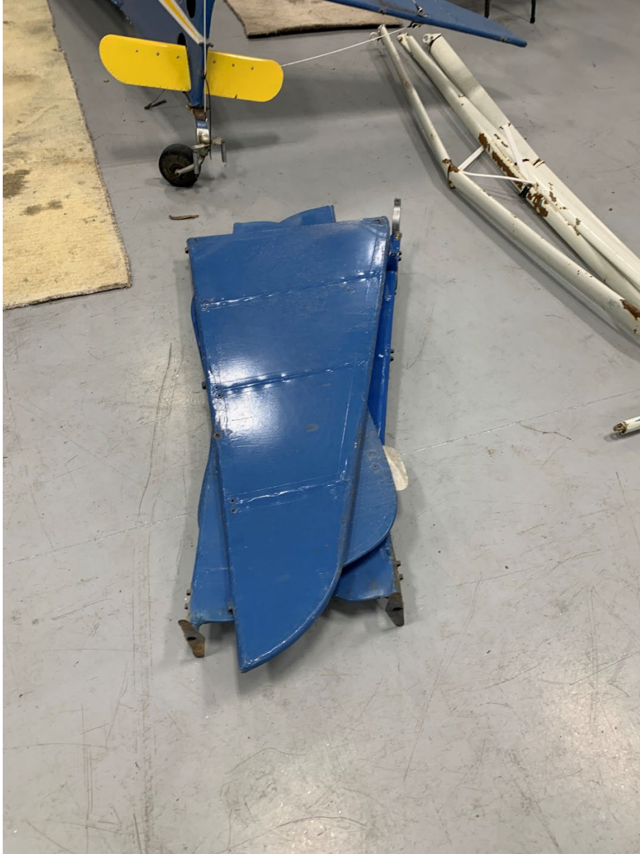
Figure 2. View of removed rudder, elevators and left horizontal stabilizer.
