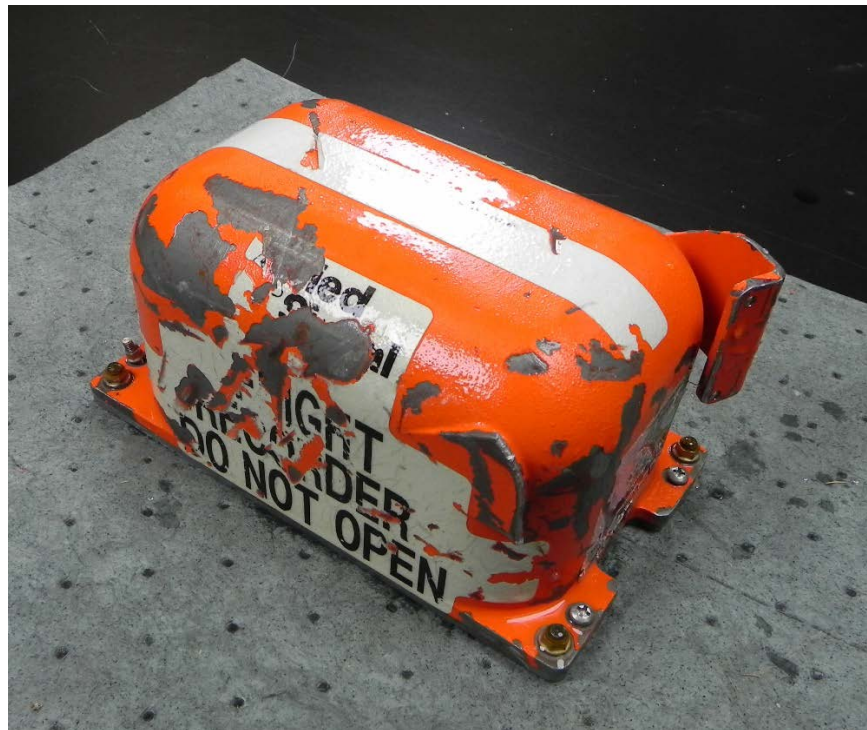
Figure 1. Damaged exterior of flight recorder.
