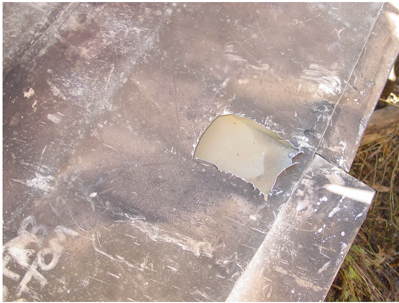
Photograph 7 (Left elevator after sample cut out)
