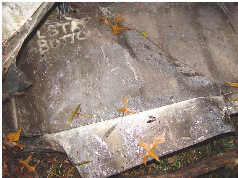
Photograph 6 (Left elevator before sample cut out)
