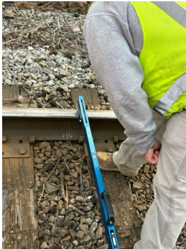
Figure 4. Investigator taking gauge and crosslevel measurements.
