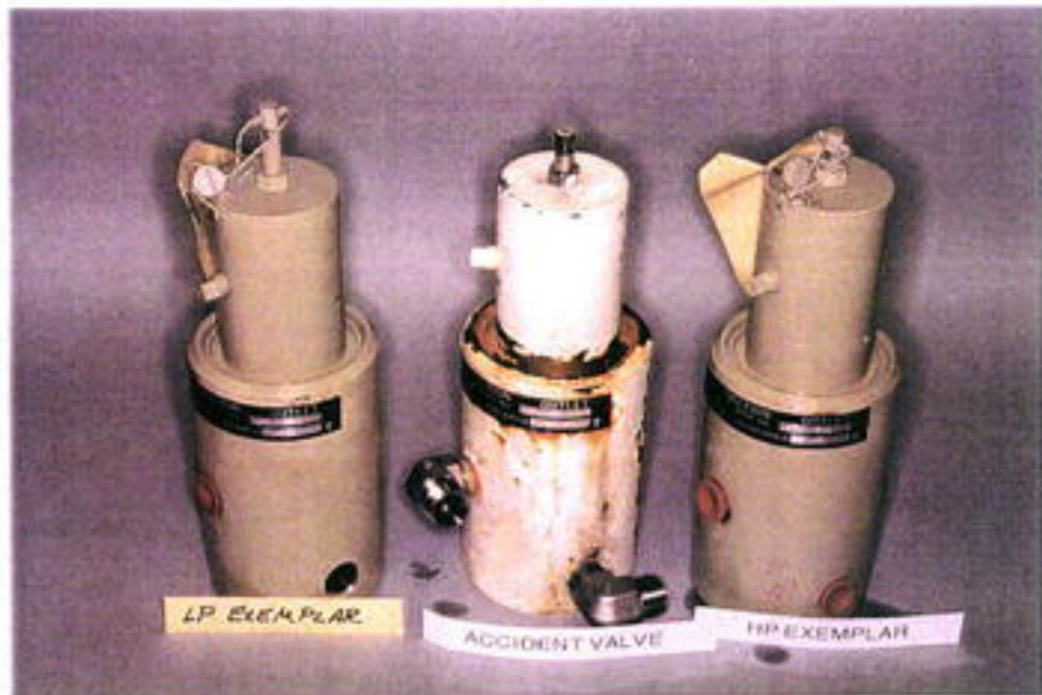
Figure 5.4 Pilot Valves Prior to Disassembly
