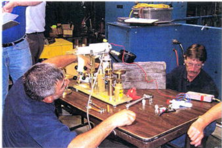
Figure 4.3 Dead Weight Test Set-up (view 2)
