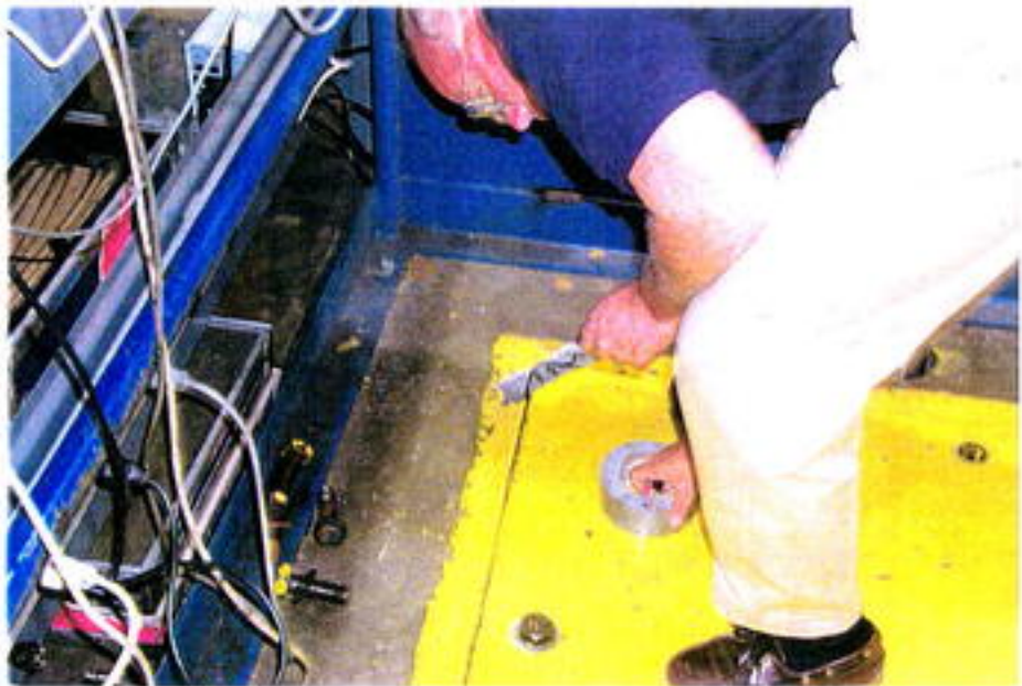
Figure 2.20 Sealing of Test Pit
