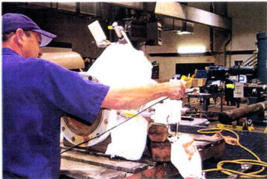
Figure 2.19 Optical Probe Inspection (View 3)
