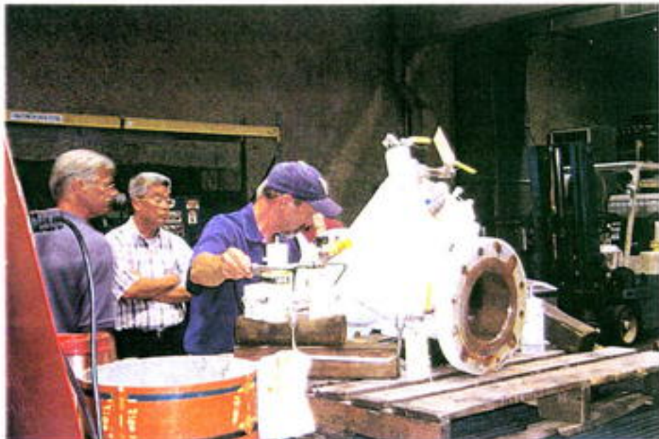
Figure 2.18 Optical Probe Inspection (View 2)
