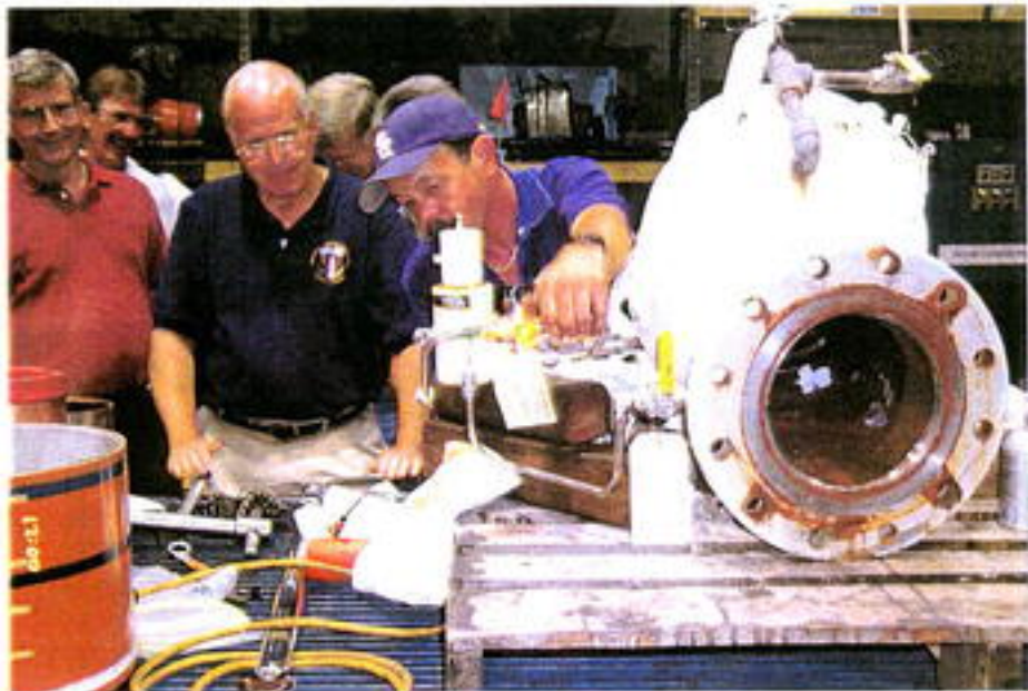
Figure 2.17 Optical Probe Inspection (View 1)
