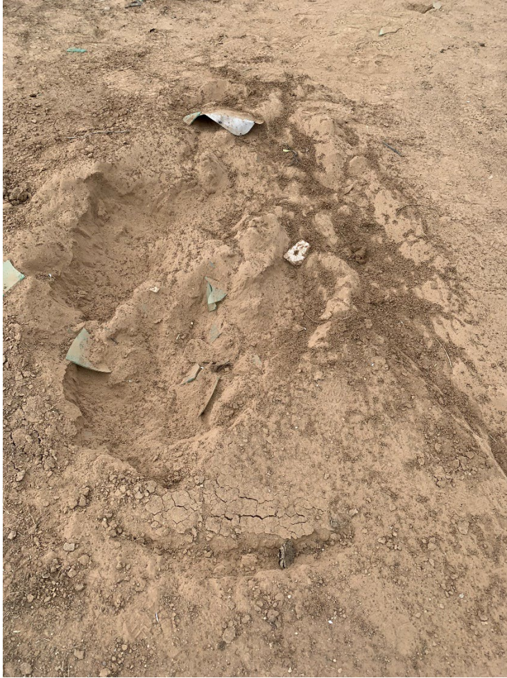
Figure 5– Impact Crater and Propeller Strike Mark
