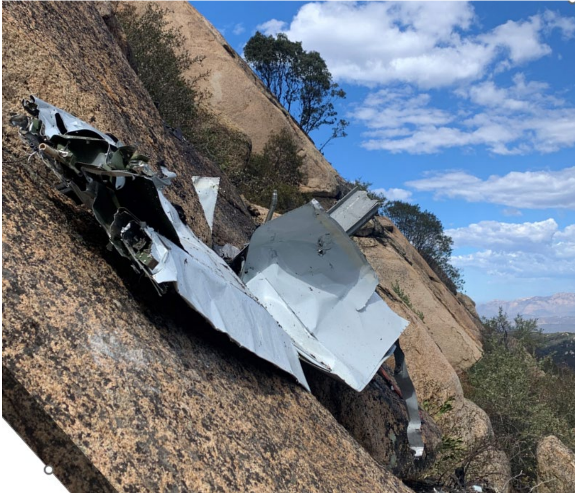
Figure 6. View of damaged wing section that came to rest on rockface
