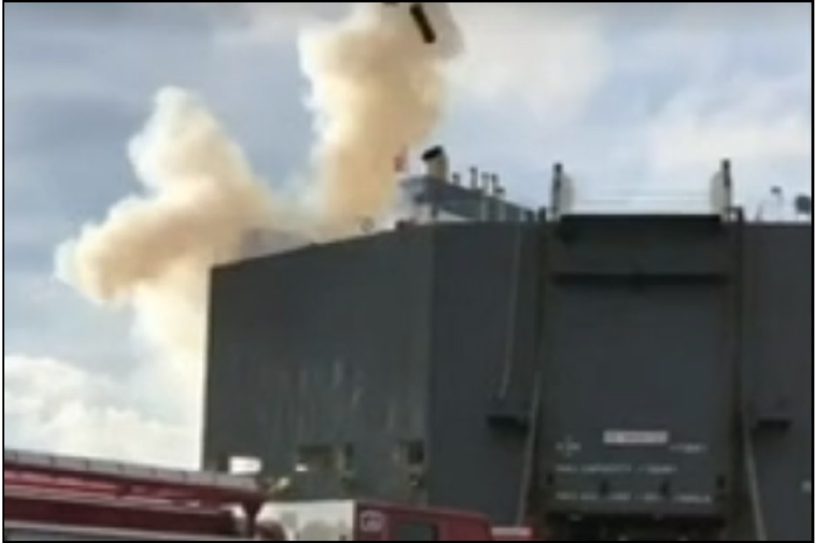
1 2 Figure 6 – Overpressurization of Deck 9 ventilation exhaust trunk (Source: WJXT)
