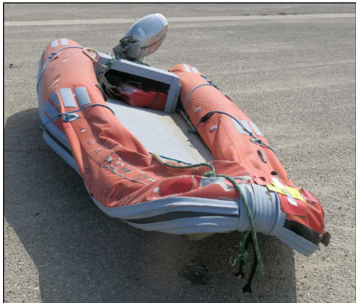
Figure 10: Postaccident photo of the skiff from the Conception . Note the cut line at the bow
