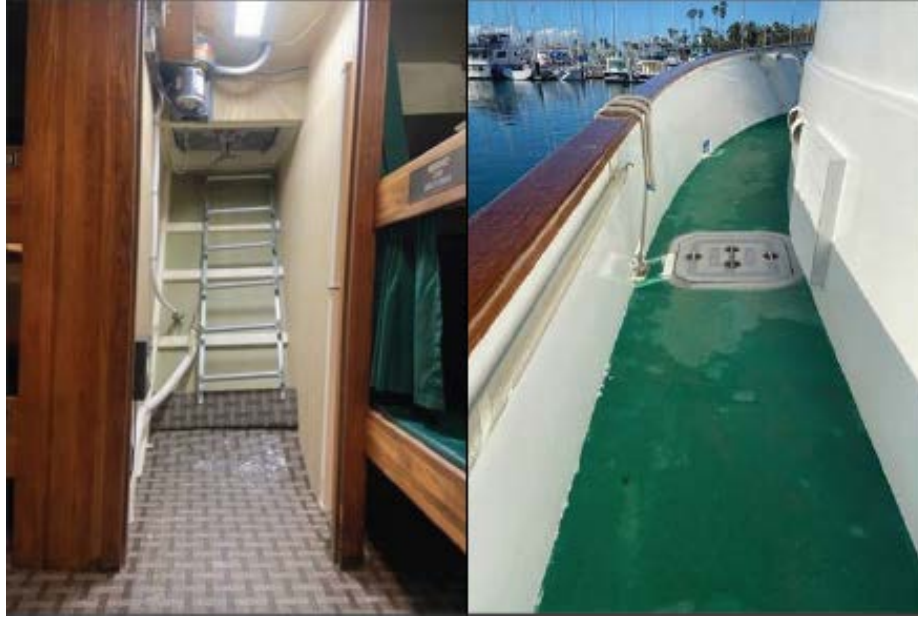
1 2 Figure 16: Modifications made to the Vision , after the accident on the Conception . Left: Ladders at 3 the forward end on each side of the bunkroom lead directly to the weather deck. Right: Flush 4 mounted watertight hatches were installed in the deck, outboard of the galley. (Source: Truth 5 Aquatics)
