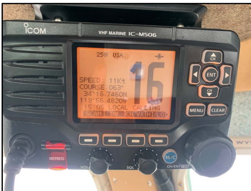
Figure 9: Conception's VHF radio located overhead in the wheelhouse. The VHF-DSC distress button in the lower left is color-coded red. (Source: B. Priddin)
