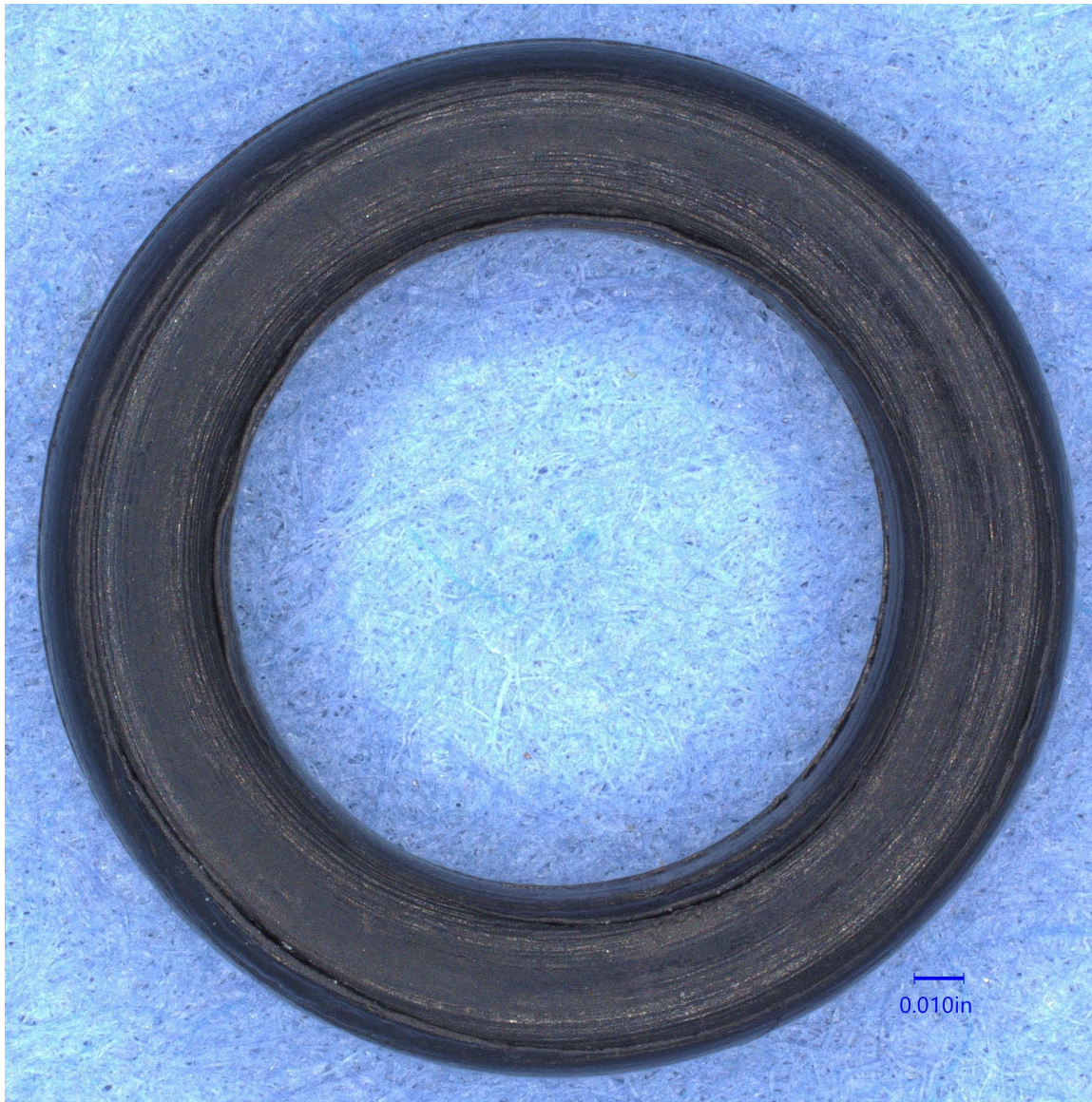
Figure 9: Example of Circumferential Splitting on Inner and Outer Diameter of the C1 Seal
