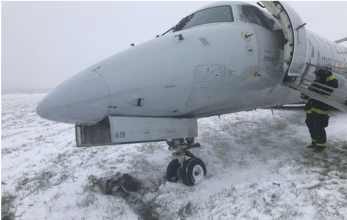
Figure 3: Nose Landing Gear Following Runway Departure
