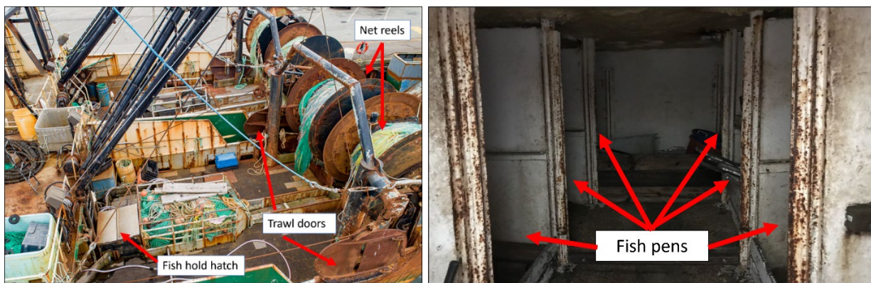
8 Figure 13. Aft working deck ( left ) and fish hold pens ( right ). (Source: Atlantic Brokerage 9 House and Marine Safety Consultants)
