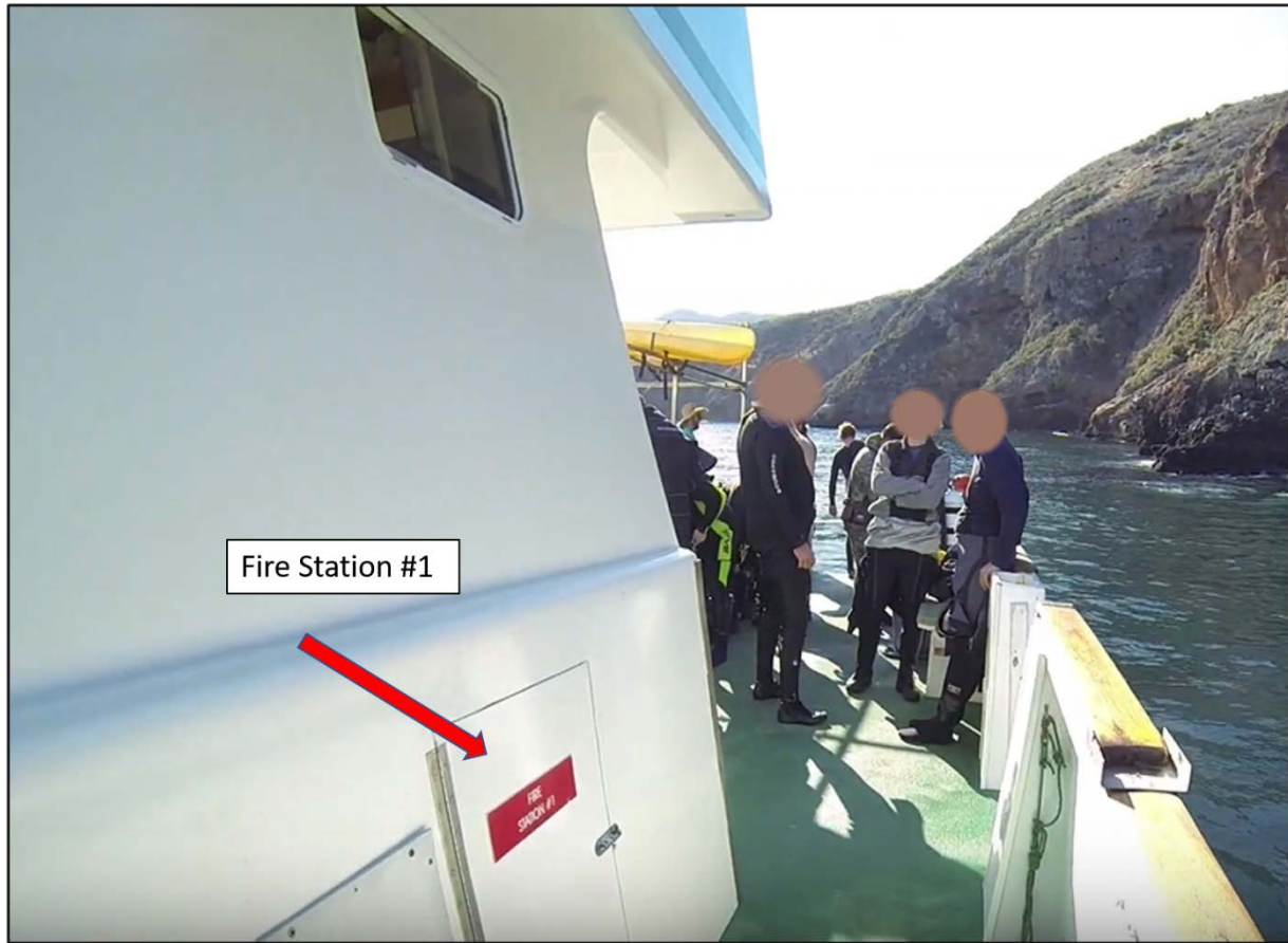
1 2 Figure 4. Fire station number one on the Conception . Located at the aft end of the galley/salon, 3 outboard on the port side, photo taken on a previous voyage (Sailor James, Youtube).
