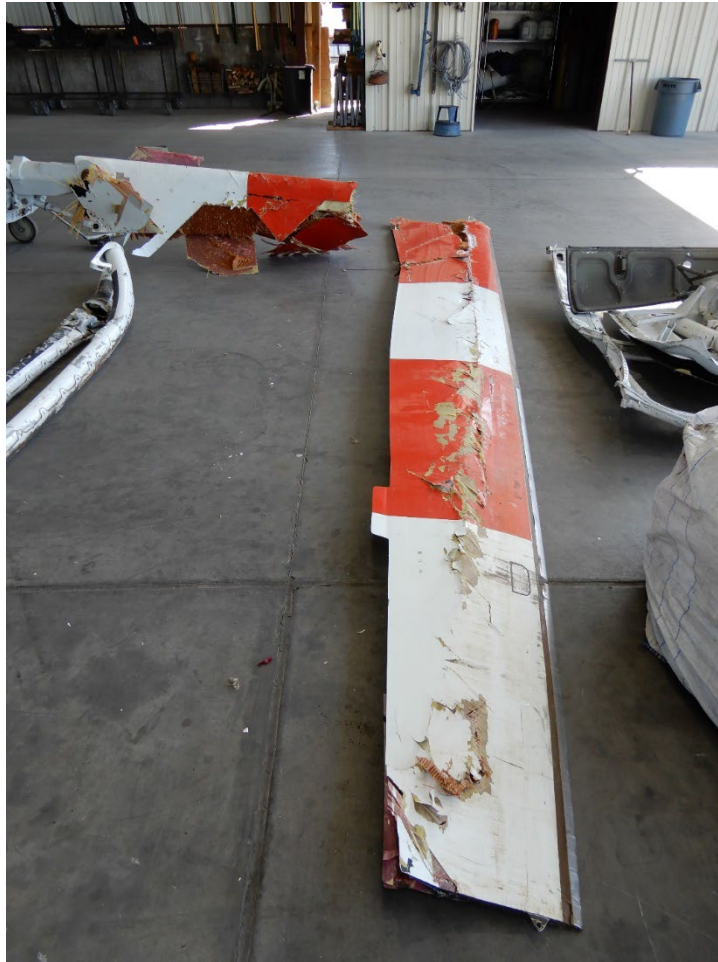
Photo 7. The white main rotor blade, top view.
