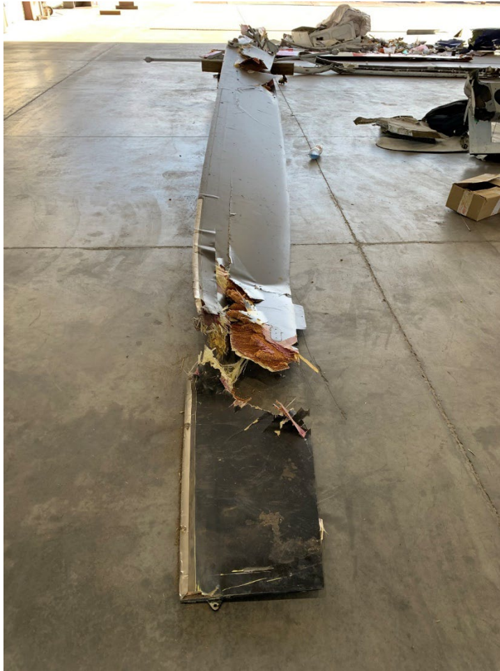
Photo 8. The red main rotor blade, underside view.
