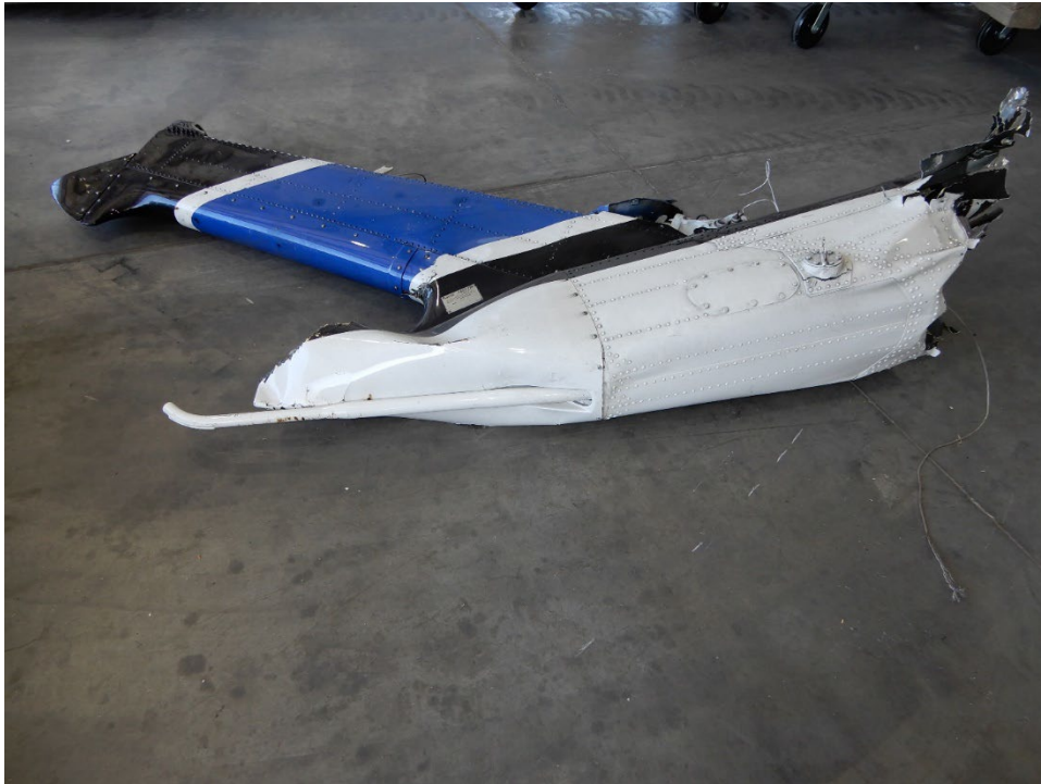
Photo 6. Vertical stabilizer without the 90° gearbox or tail rotor assembly.
