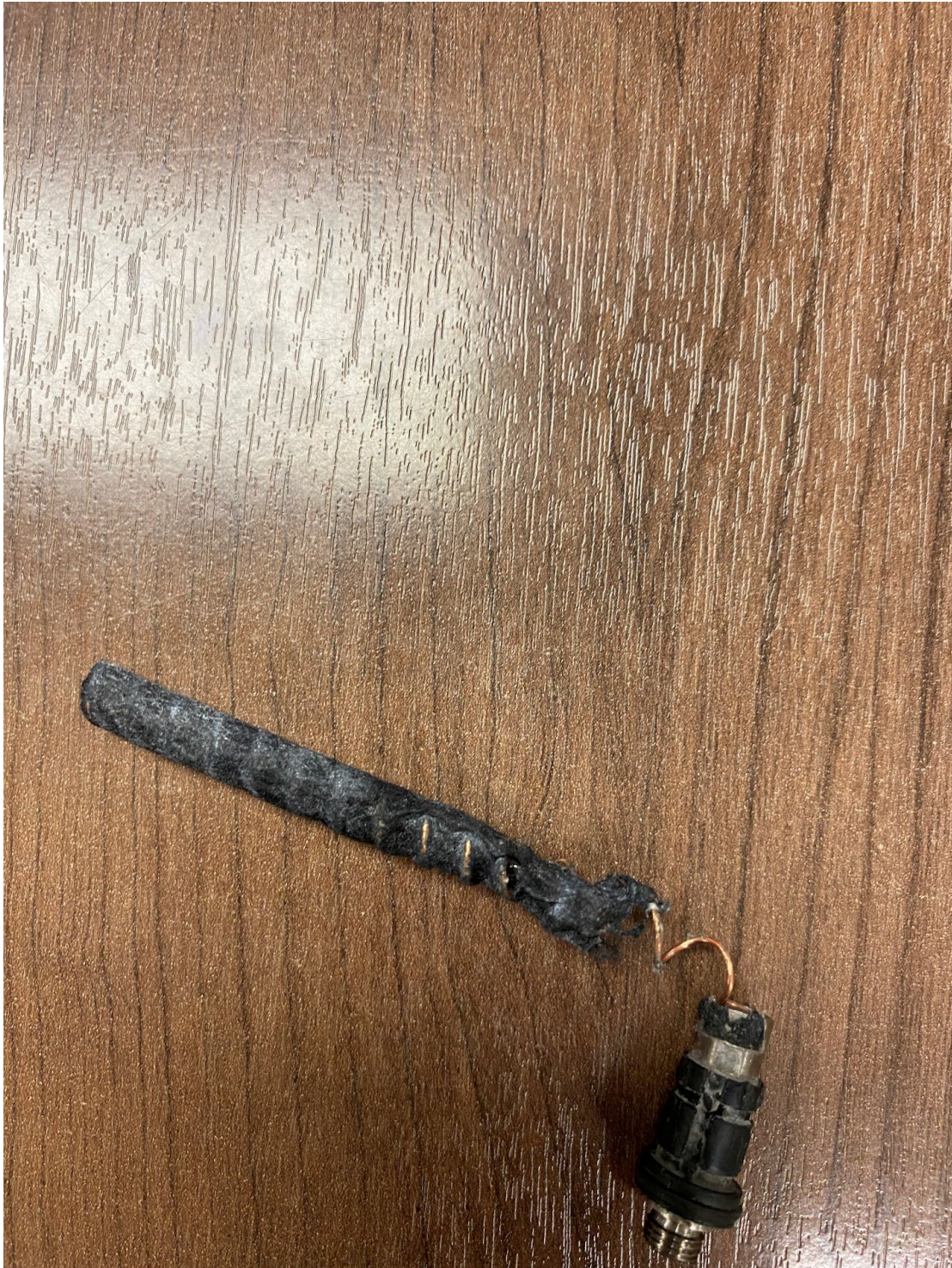
Antenna base with copper coil and wrap removed from handheld radio
