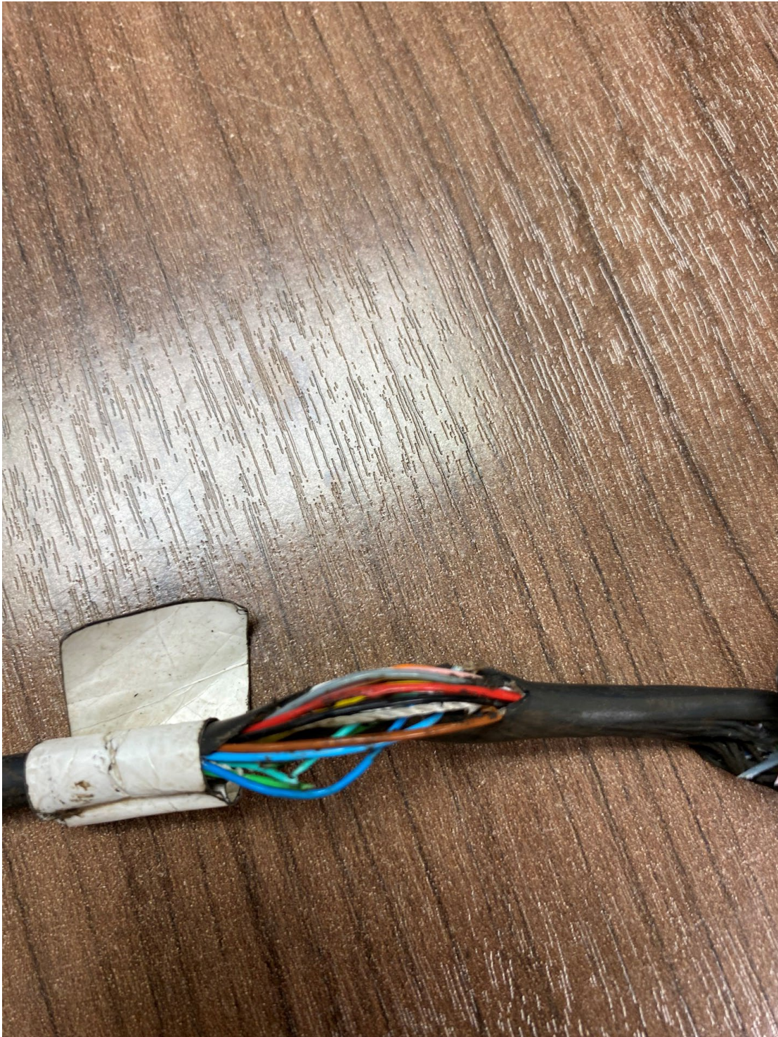
Severed cables of microphone cord
