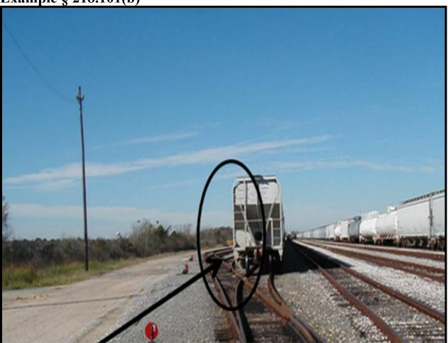
These cars are fouling the adjacent track, and are past the clearance point noted in the railroad operating rules. This noncompliance should be recorded under §218.101 (b).
