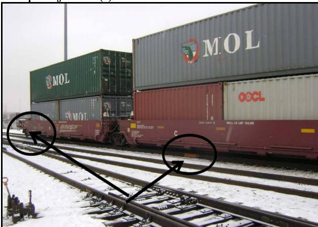
These cars are <u>NOT</u> fouling the adjacent track, but they are past the clearance point noted in the railroad operating rules. This non-compliance should be recorded under §218.101 (a).
