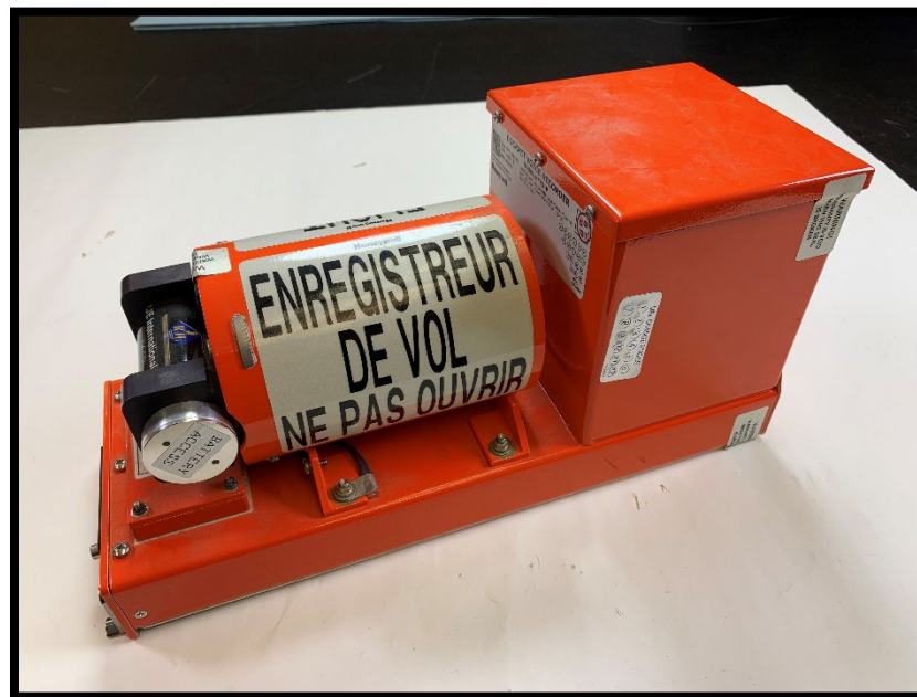
Figure 1. Condition of CVR, as received.
