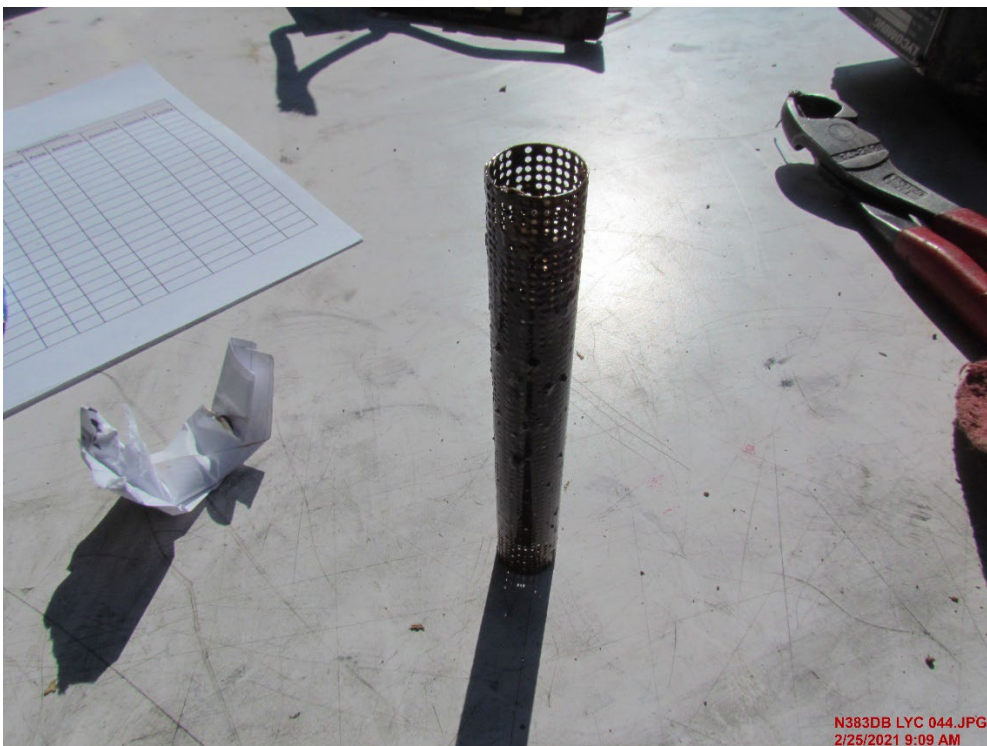
Figure 24- Oil suction screen (Courtesy of Lycoming).
