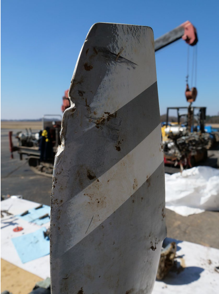
Figure 28-Leading edge damage to propeller blade
