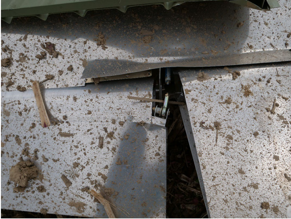
Figure 8- Right flap push/pull rod, broken.
