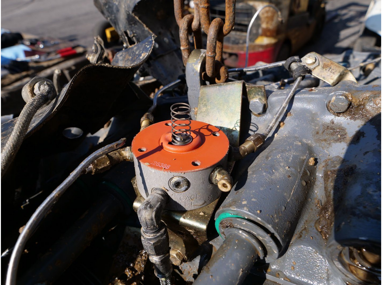
Figure 19 - Fuel flow divider diaphragm, note tear on left side of spring.
