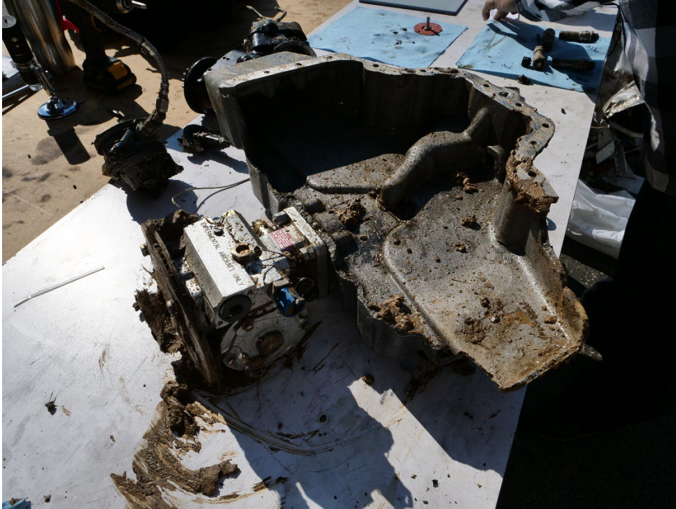
Figure 23- Oil sump, fractured.
