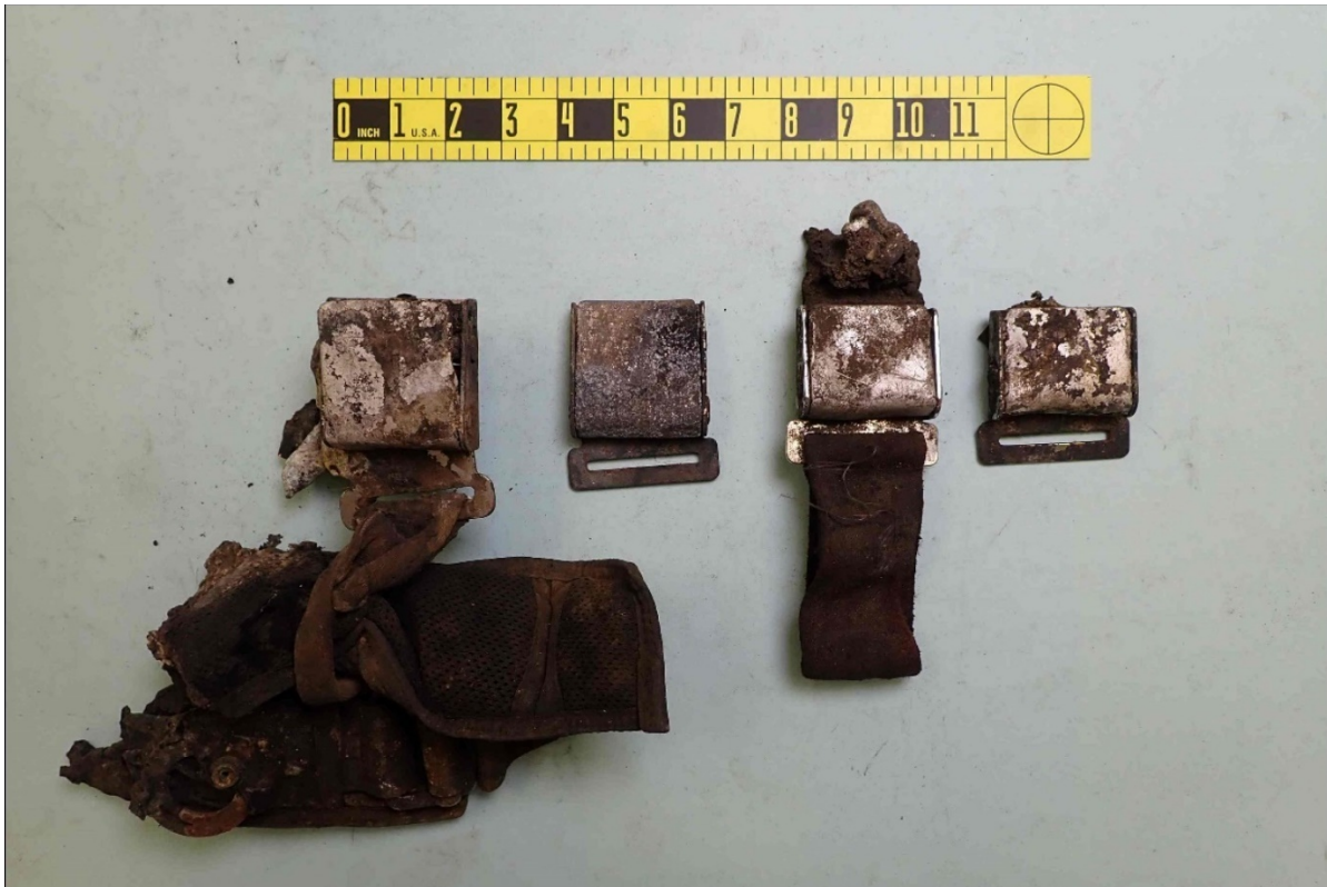
Photo 5: Latched Bench Seat Buckles, with a Parachute Harness Still Attached to the Left Buckle
