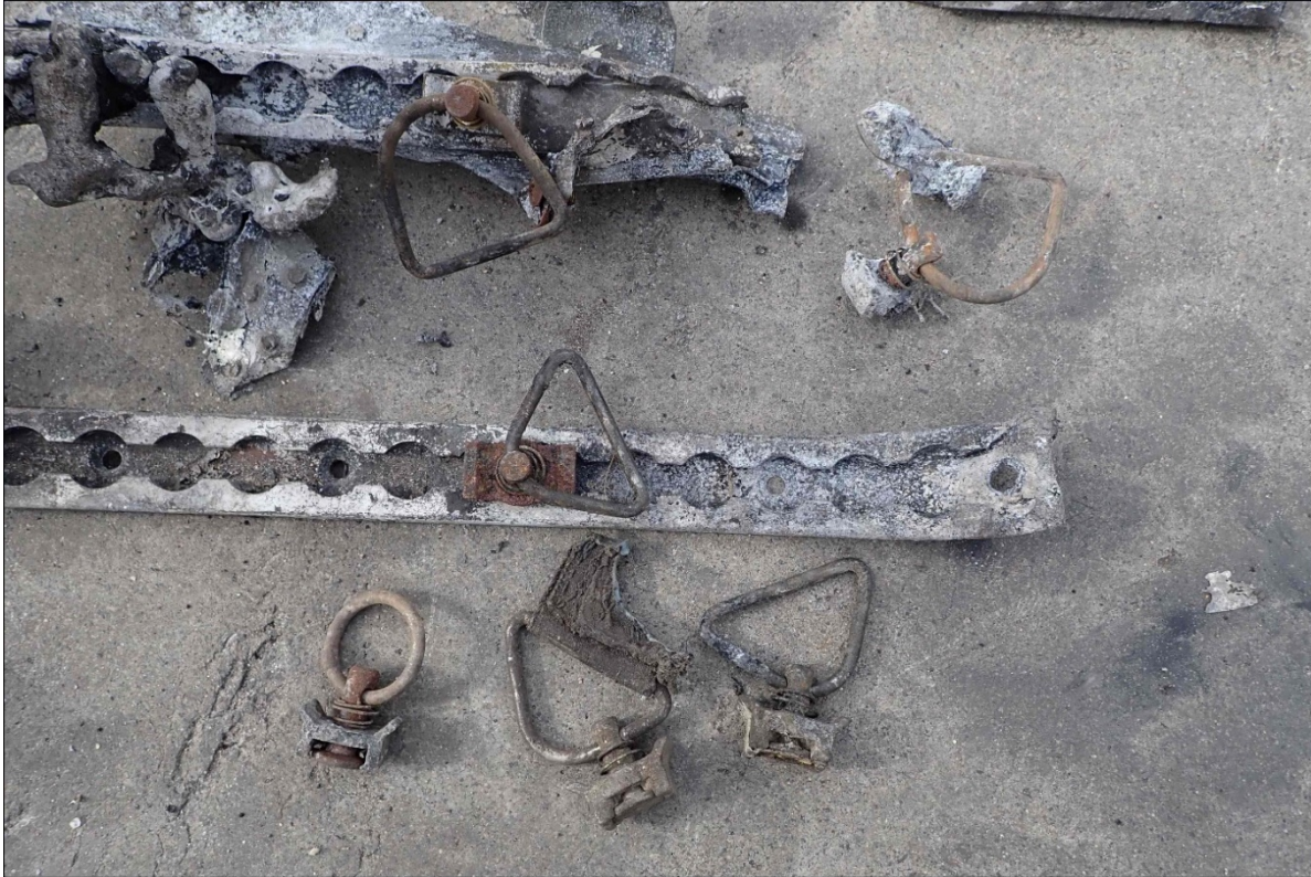
Photo 8: Undamaged Tethering Rings
