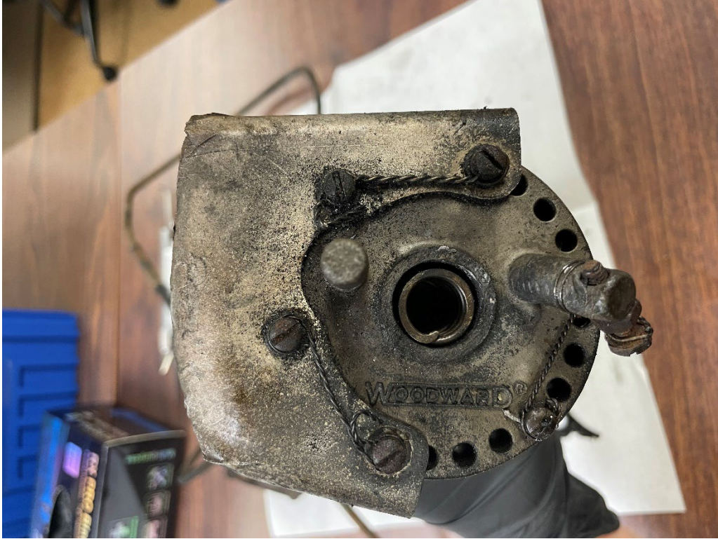
Figure 4: View of the Top of the Governor Showing The Fractured Governor Assembly Cover.
