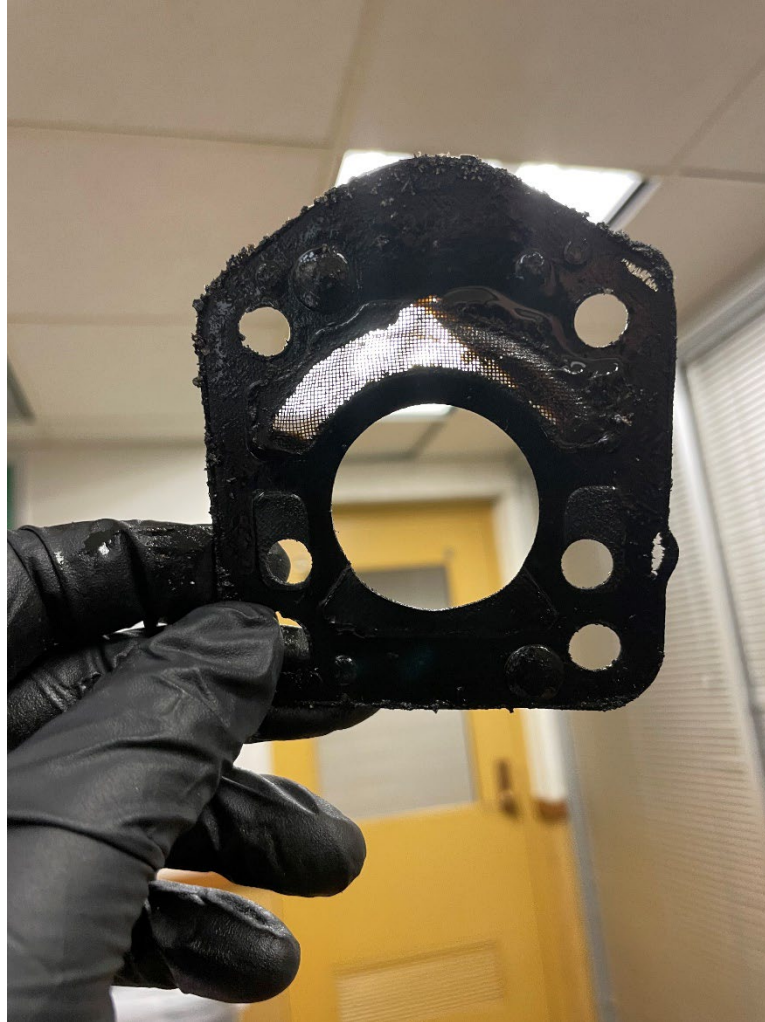
Figure 5: View of the Governor Base Gasket. Note the Coked Oil.
