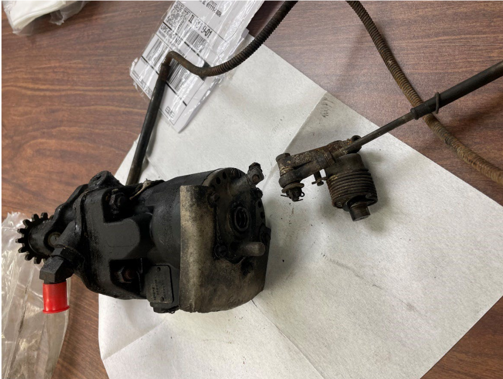
Figure 3: Propeller Governor as Received. Note the Overall Heat Damage and Impact Damage to the Cover.
