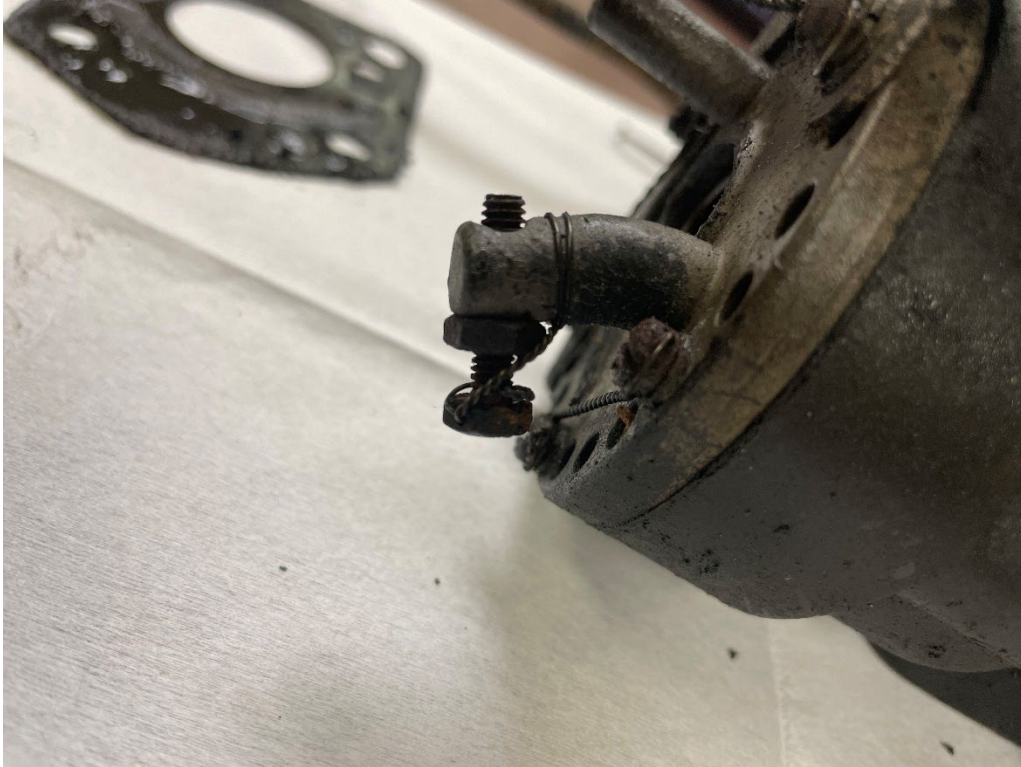
Figure 6: View Showing the bent maximum speed adjustment post the maximum adjustment speed screw had 3 threads showing.
