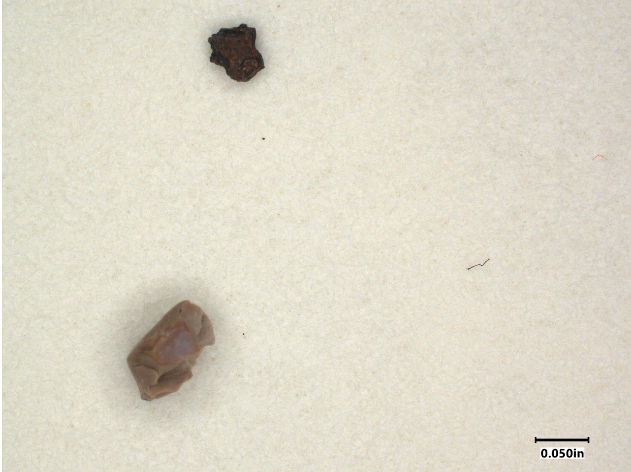
Figure 3: NTSB Digital Photograph. View of Both Pieces of Contamination With Scale.
