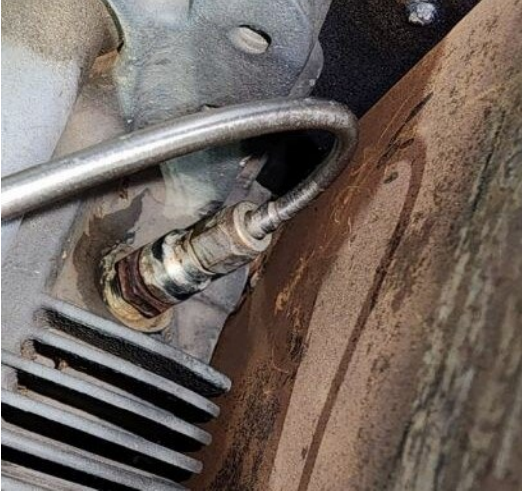
Figure 3: Digital Photograph From Lycoming. View Showing Leakage From Fuel Injector Nozzle During Engine Operation Testing without an Insert or Restrictor Installed.
