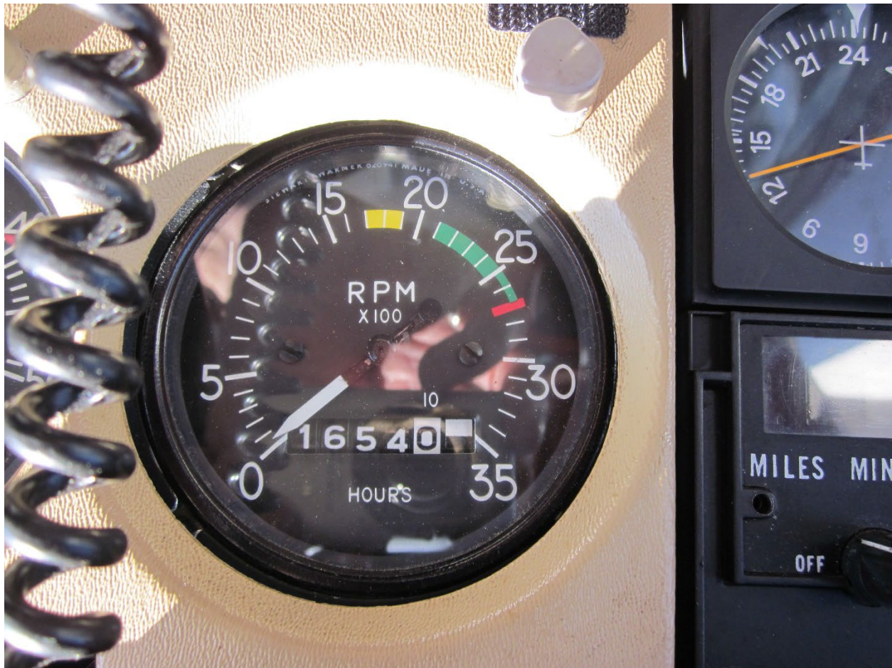
Figure 6: FAA Digital Photograph. View of the Tachometer Taken PostAccident. Note the reading 1,654.0.
