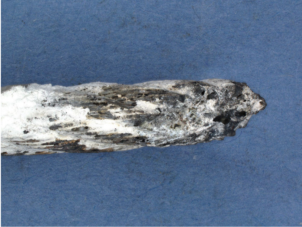
Figure 3: NTSB Materials Laboratory Photograph of One End of the “Debris End” of The Fractured Aileron Cable Assembly with the Profile Rotated 90°. View at 20X magnification.
