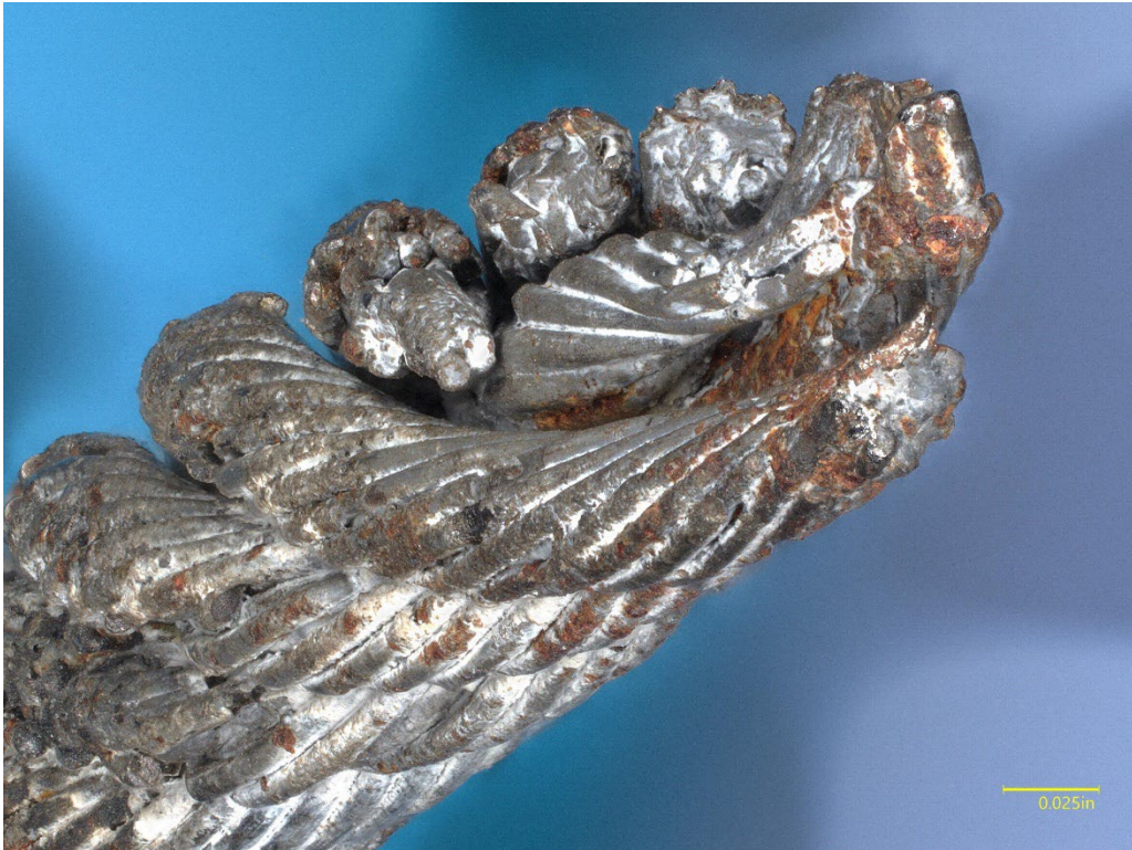
Figure 4: NTSB Materials Laboratory Photograph of the Fitting End of the Fractured Aileron Cable Assembly After Cleaning. View at 40X magnification.
