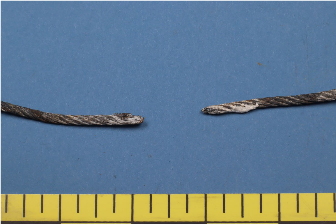
Figure 2: NTSB Materials Laboratory Photograph of Aileron Cable Assembly Received Showing the Fractured Section in Question.
