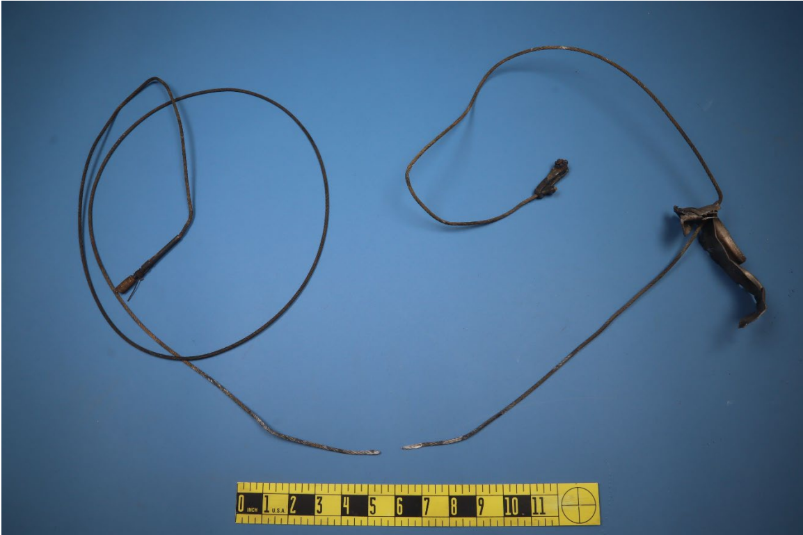
Figure 1: NTSB Materials Laboratory Photograph of Aileron Cable Assembly Received. The Fractured Section is Seen in the Lower portion of the Photograph adjacent to the ruler.
