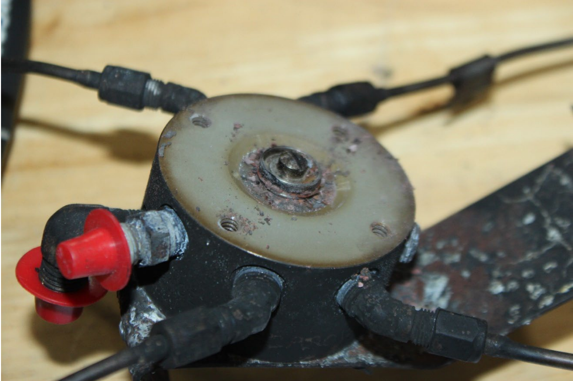
Figure 7: View of the Spool in the Fully Closed Position.
