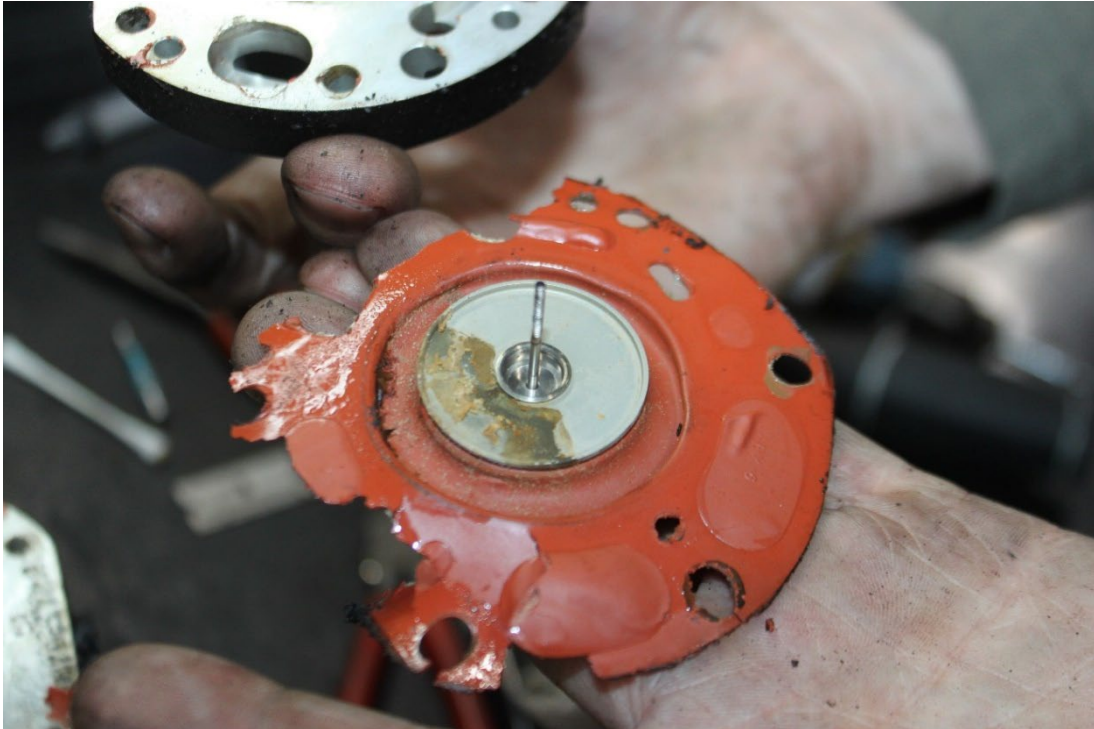
Figure 14: View of the Unmetered side of the Fuel Diaphragm showing Contamination.
