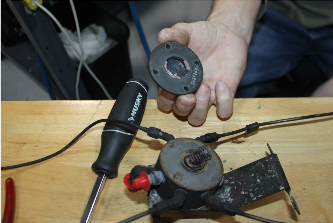
Figure 6: View of the Manifold Valve Following Removal of the Cover. Note the Heat Destroyed Diaphragm.
