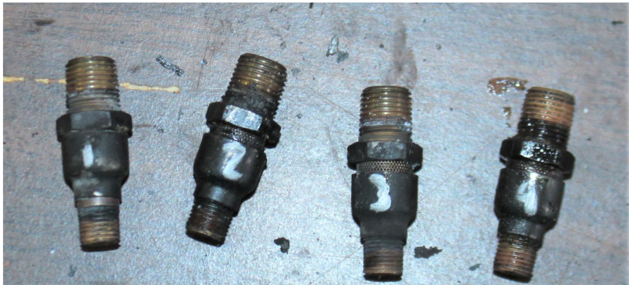
Figure 1: Close-up Examination of the Fuel Injector Nozzles After Removal from Engine. Note the lack of an insert or restrictor on the lower portion of each nozzle.
