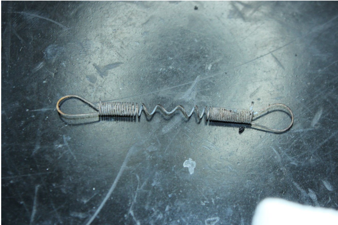
Figure 18: View Showing the Distortion of the Mixture Control Clevis Spring.
