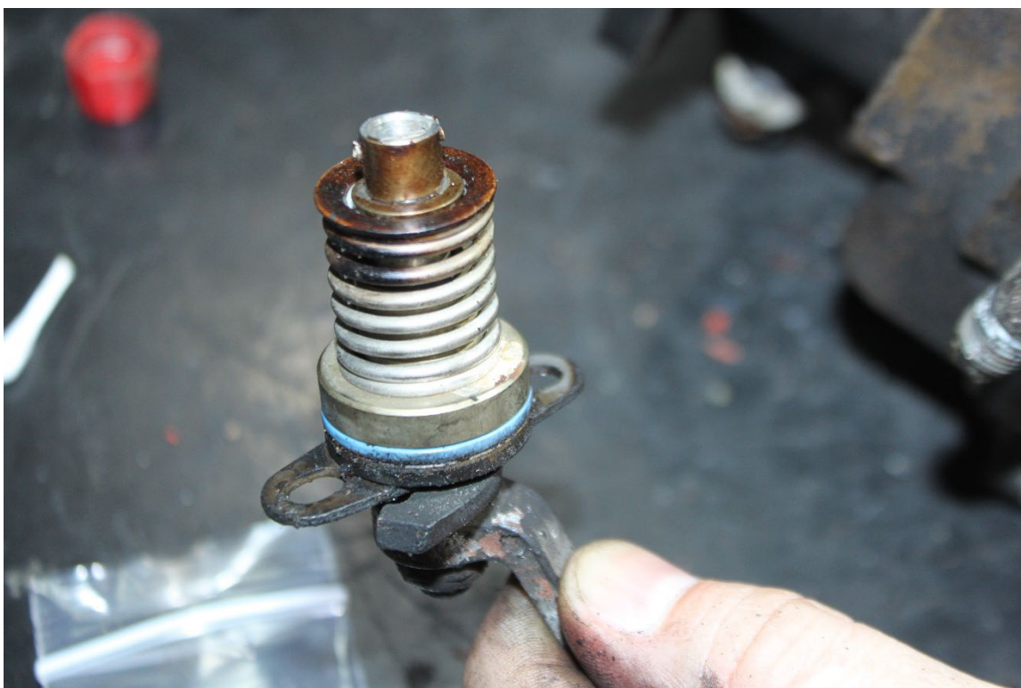
Figure 17: View Showing the Contamination on the Mixture Control Bushing.
