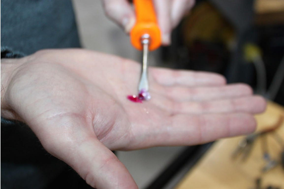
Figure 9: View of the Liquid Drained From the No. 4 Fuel Injector Line and the Positive Results when Tested with Water Finding Paste.
