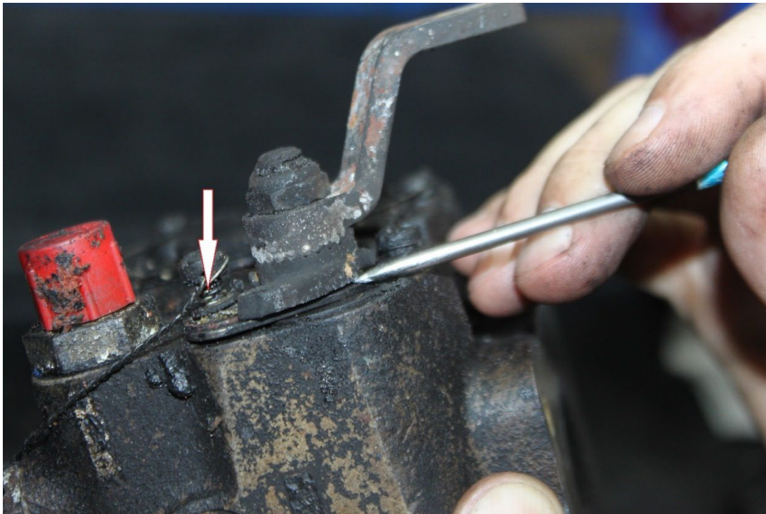
Figure 16: Arrow Points to Where Missing Mixture Control Nylon Stop Would be Installed.
