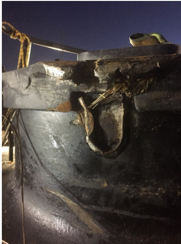
Figure 3: GATX 90208: missing swing bolt on manway (photograph courtesy of Union Pacific Railroad)
