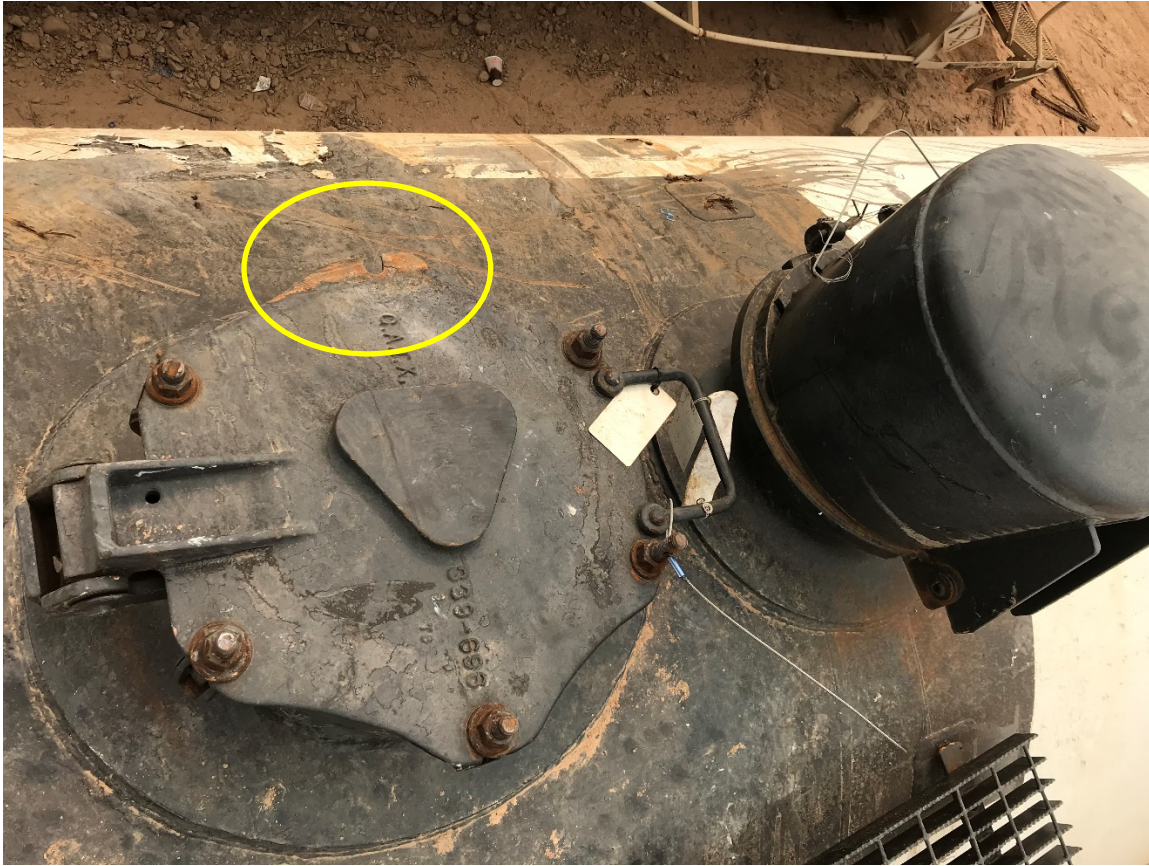
Figure 1: GATX 90208 PRD housing and manway with a missing bolt (circled yellow) (photograph courtesy of FRA)
