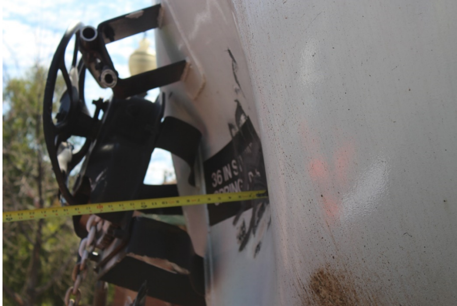
Figure 7: GATX 1384: Dent on the B-end head (photograph courtesy of PHMSA)
