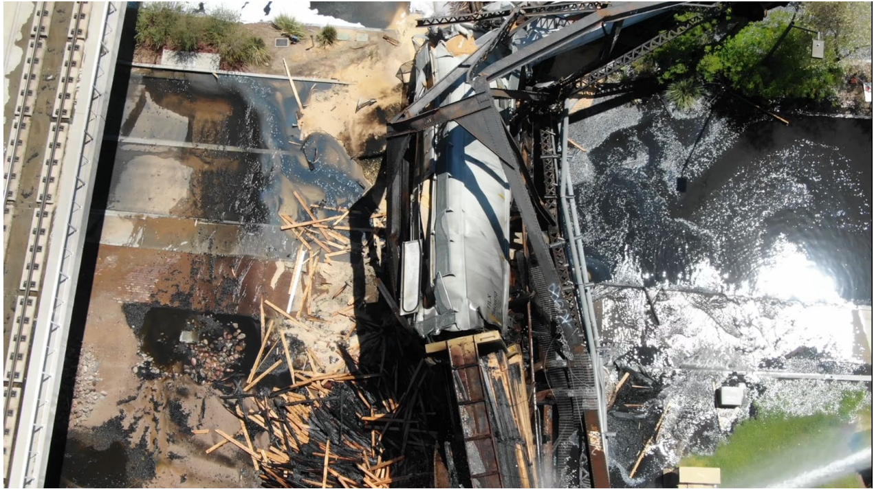
Figure 2: Aerial view of burned lumber car TTZX 862290 in front of soybean car TILX 540850
