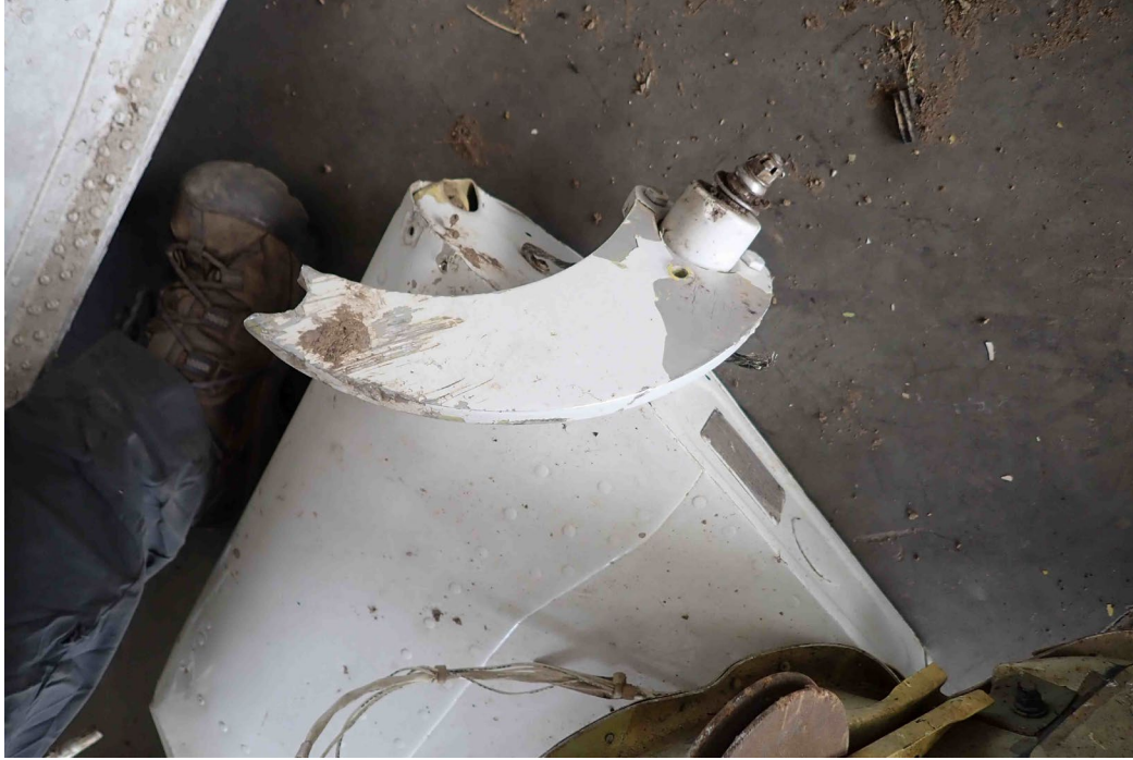
Photo 40 - Elevator control horn
