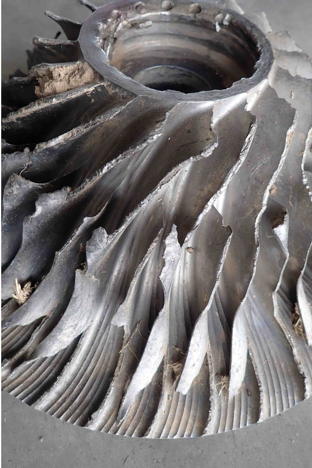
Photo 57- Number 2 high pressure compressor
