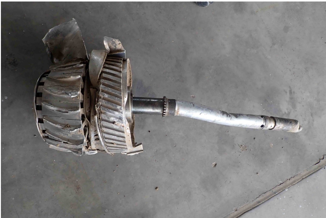
Photo 51 – Number 2 low compressor fan fragments
