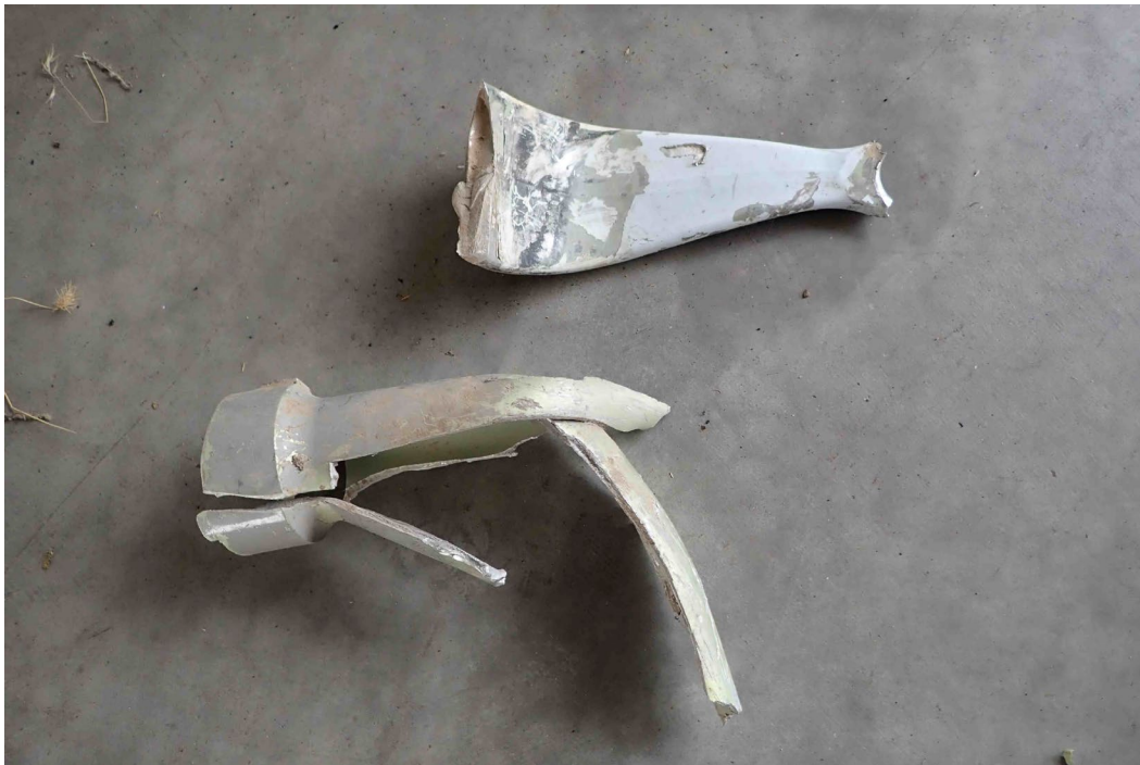
Photo 29 – Nose landing gear fragments
