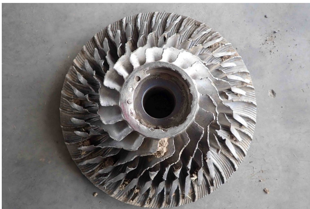
Photo 56 – Number 2 high pressure compressor
