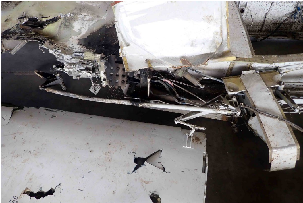
Photo 31 - Left wing flap control system
