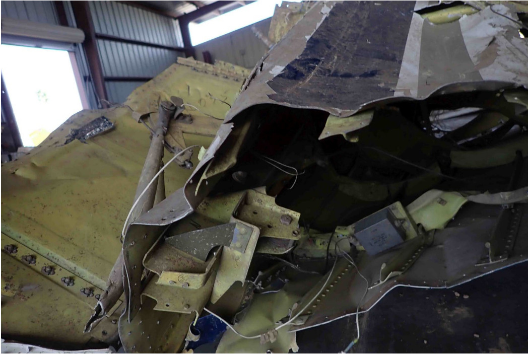
Photo 38 – Elevator aft bellcrank
