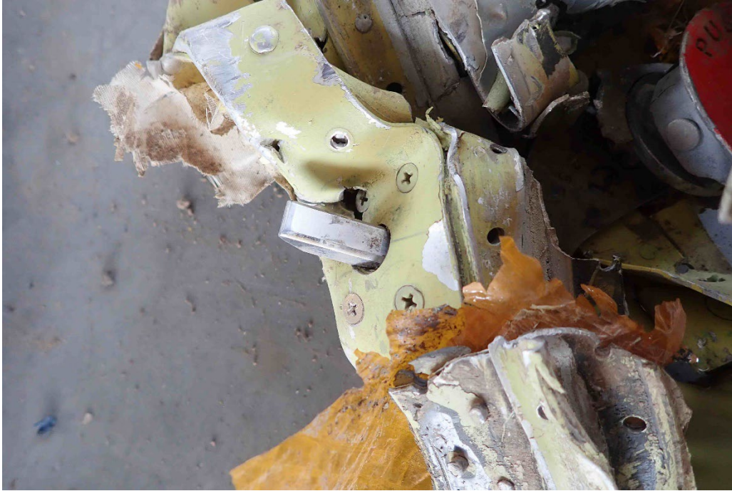
Photo 12 – Emergency door lock pin
