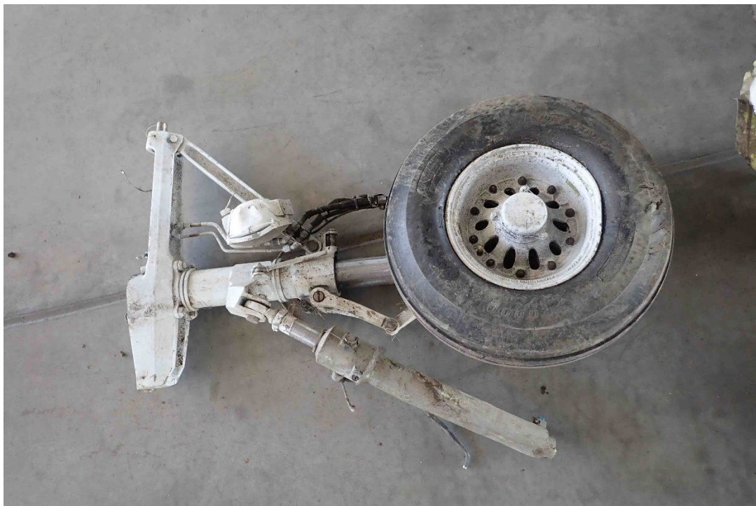
Photo 27 – Left main landing gear assembly
