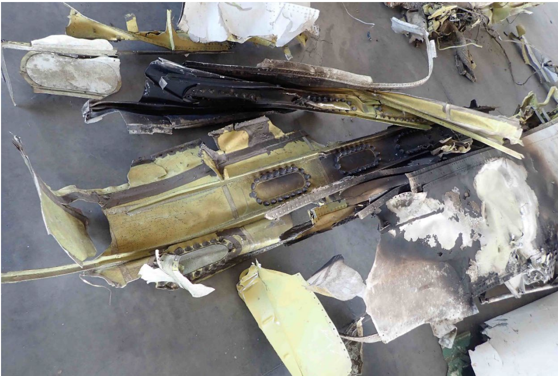
Photo 21 – Left wing leading edge fuel tank
