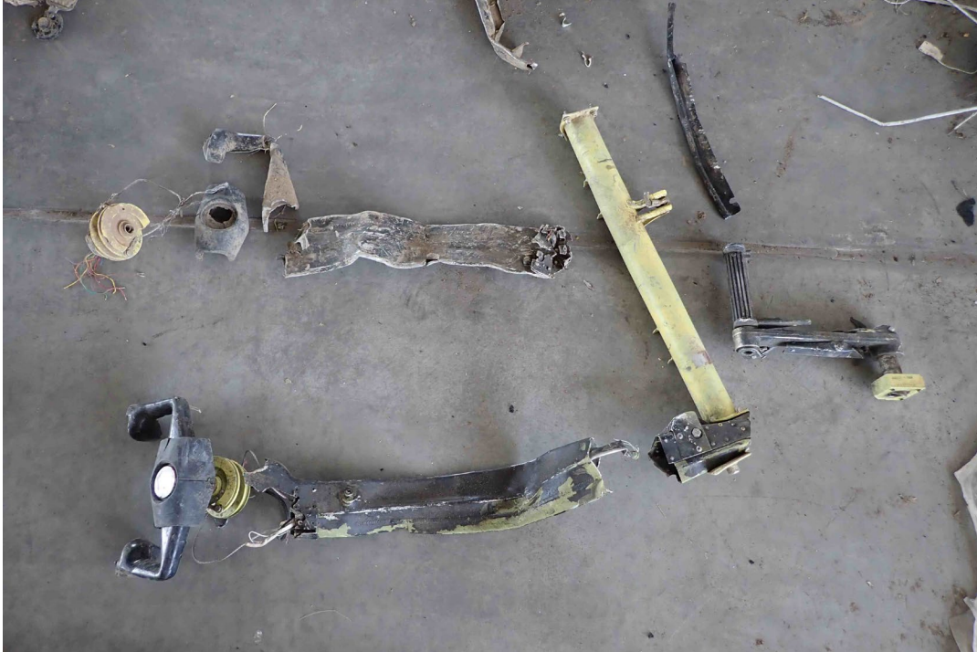
Photo 32 - Fragmented remnants of both control columns
