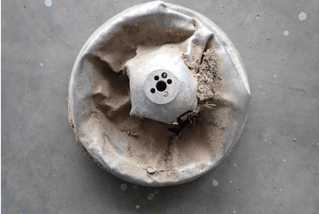
Photo 53 – Number 2 engine inlet cone
