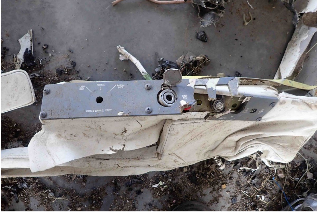
Photo 42 – Oxygen control panel
