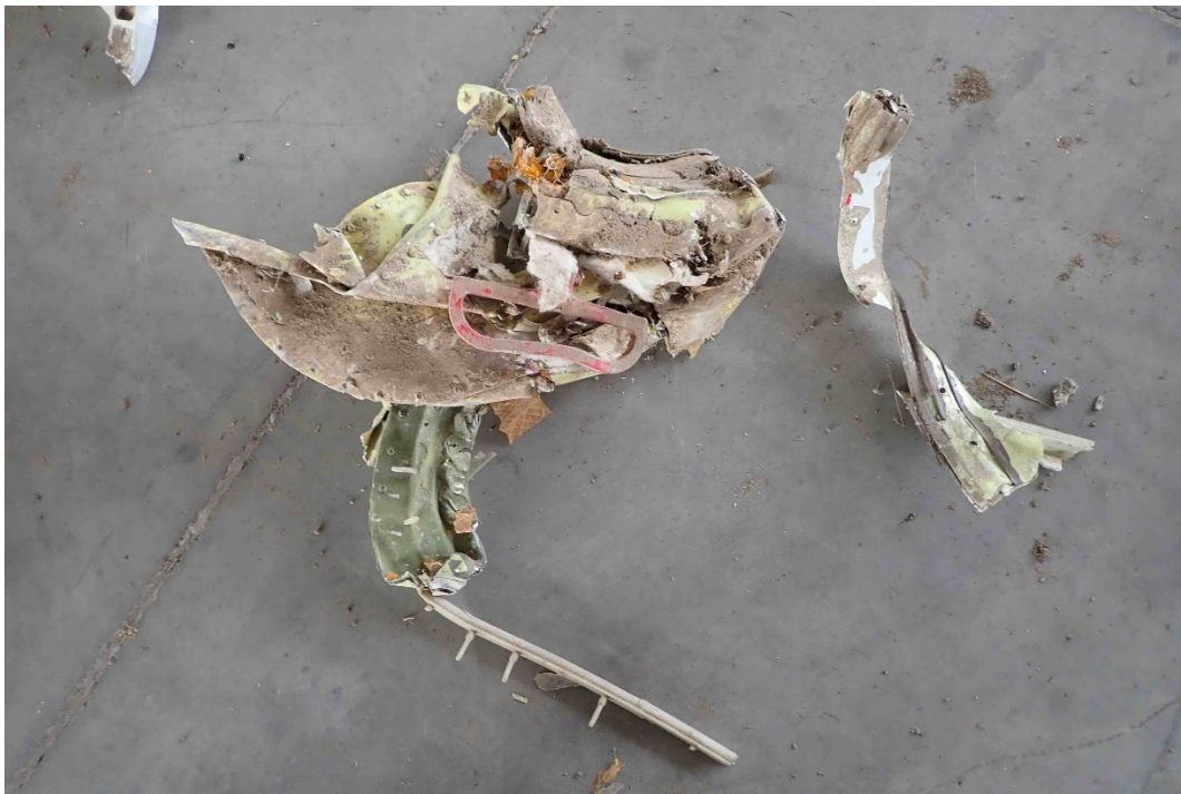
Photo 13 – Emergency door frame
