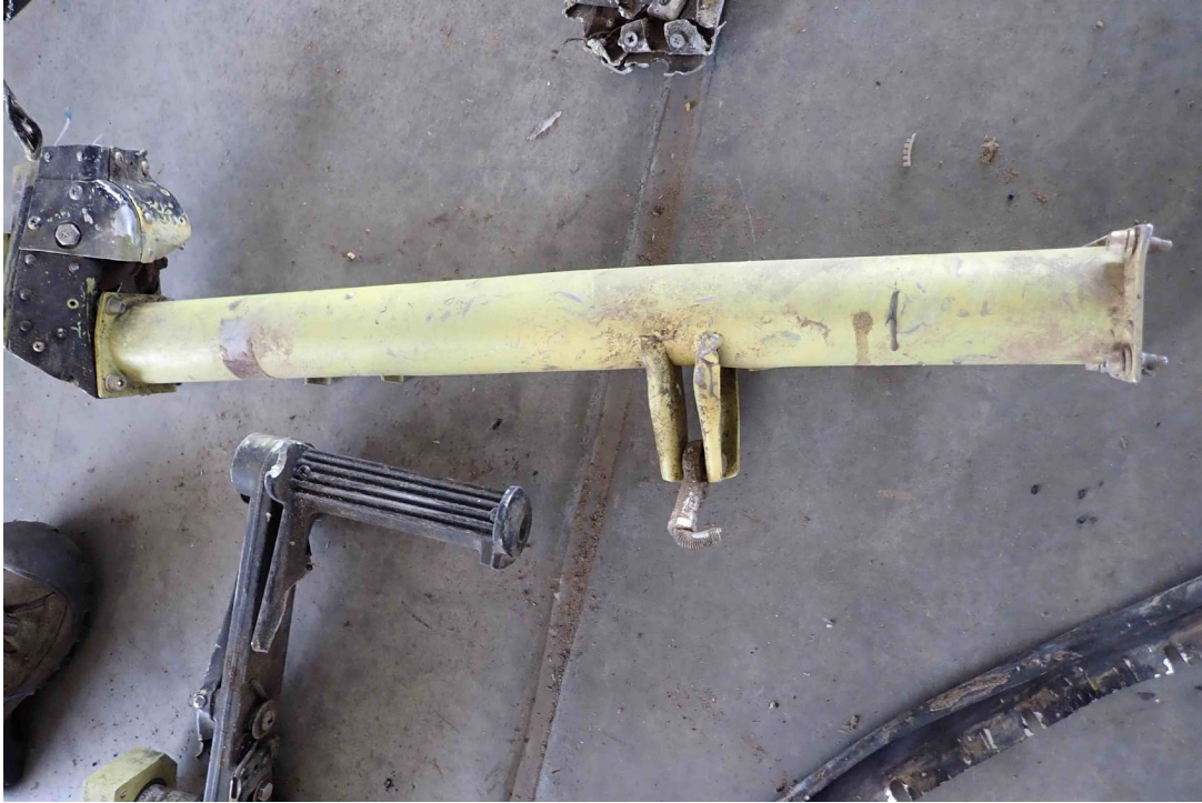
Photo 36 - Elevator control assembly
