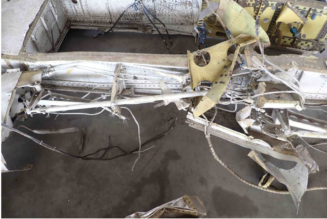
Photo 30 – Left wing flap control system
