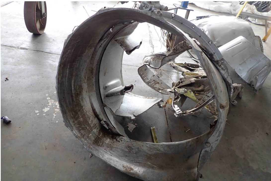
Photo 47 – Number 1 engine low compressor fan shroud
