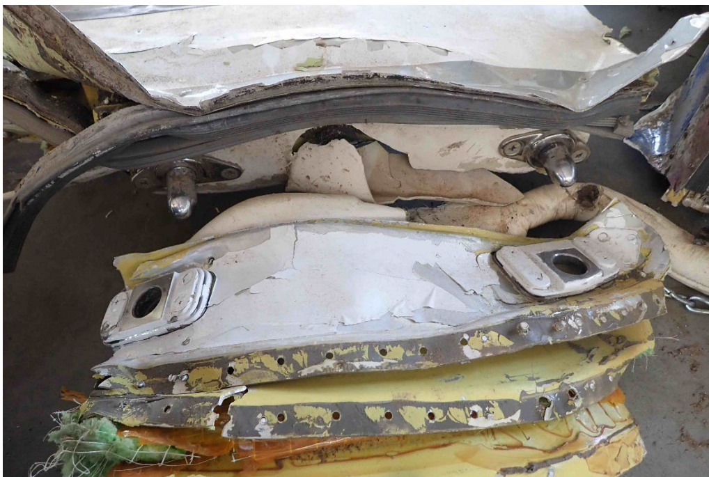
Photo 6 – Left side door lock pins and holes
