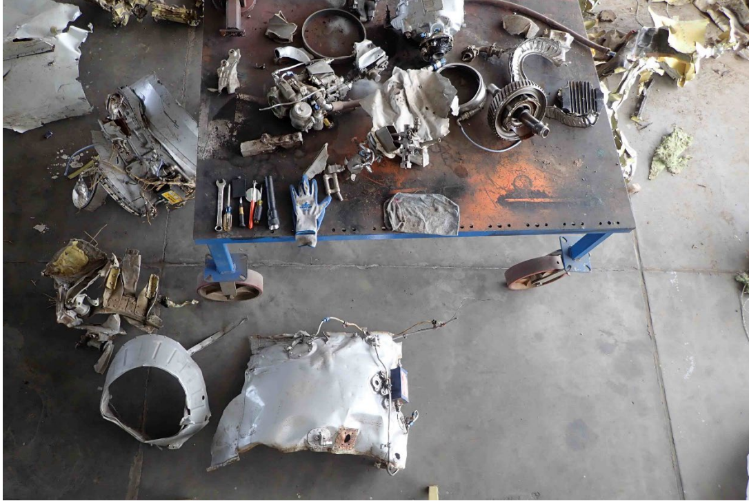
Photo 44 – Number 1 engine remnants
