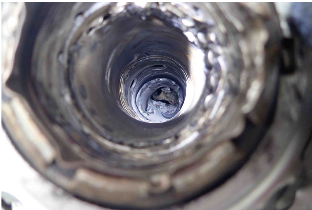
Photo 55 – Number 2 drive shaft that connects the booster assembly to the low turbine wheel
